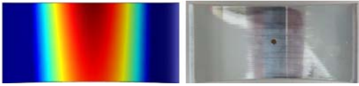
Figure 12: Comparison of calculated wear pattern and the resulting wear pattern of a conducted test.
