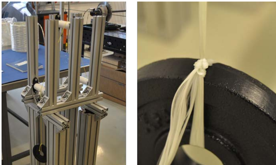
Figure 3: Test setup for manual spreading (left) and knot to connect the fibre bundle to the stress inducing weights (right).
