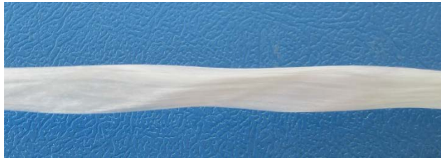
Figure 2: Detailed view on the StarRov 086 direct E-glass roving covering a length of approximately 50\text{mm} .
