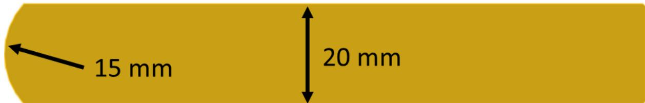
Figure 5: Sketch of the load-transferring indenter; the full length of this component is 125 mm with a diameter of 20 mm and a curvature at the tip of a 15 mm radius.
