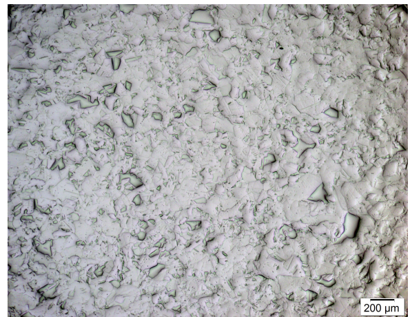
Figure 4.4: Image of the microstructure of Co.
