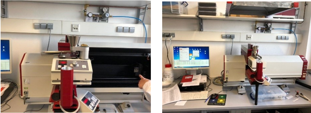
Figure 2. 7: LD machine Helos/KR at Helmholtz Institute Freiberg
