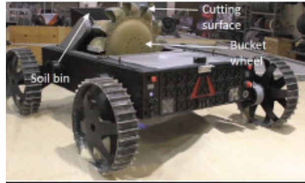
Figure 8.6: Bucket-wheel excavator with a bucket wheel in the middle [32]
