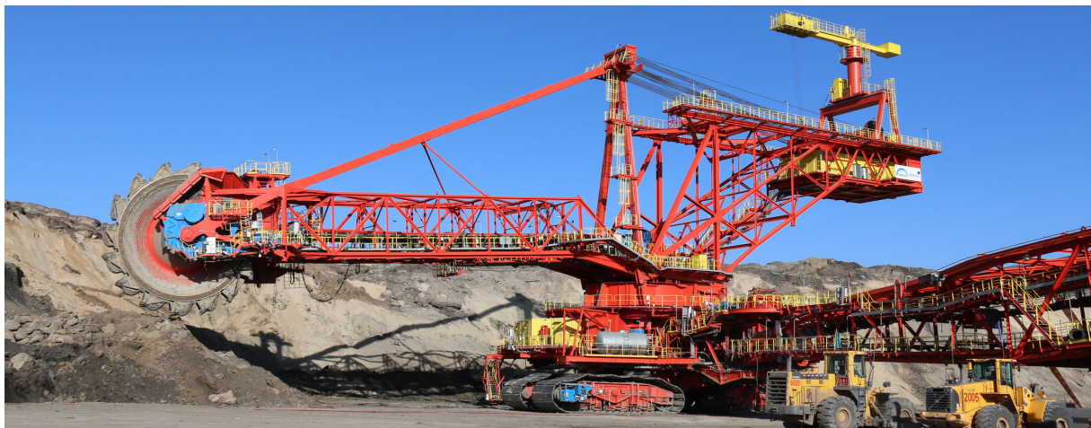
Figure 8.4: Bucket-wheel excavator for coal mining [55]
