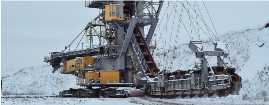
Figure 8.14: Bucket chain excavator [54]
