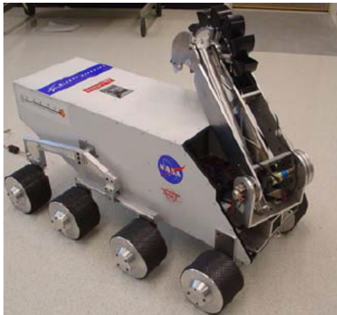
Figure 8.5: Lunar excavator by the Colorado School of Mines [15]
