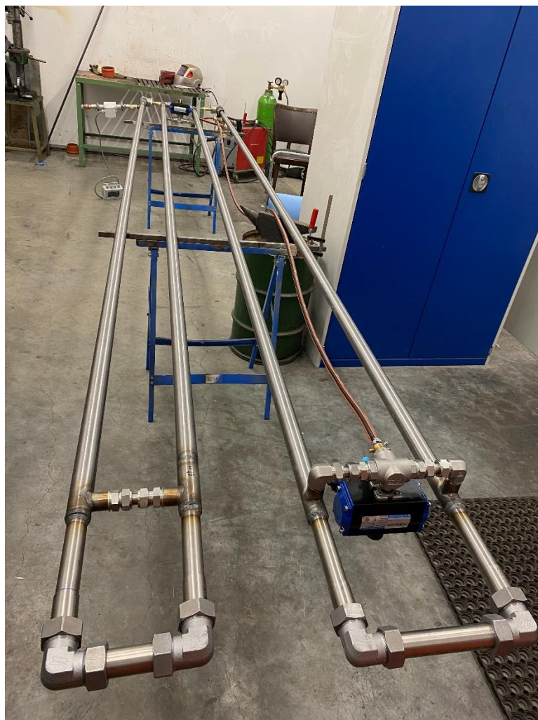
Figure 35: Pipe arrangement of the HX at the testing facility
