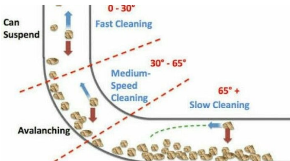
Figure 5: Guidelines for effective hole cleaning (Abdelaziz Gabr, 2017)
