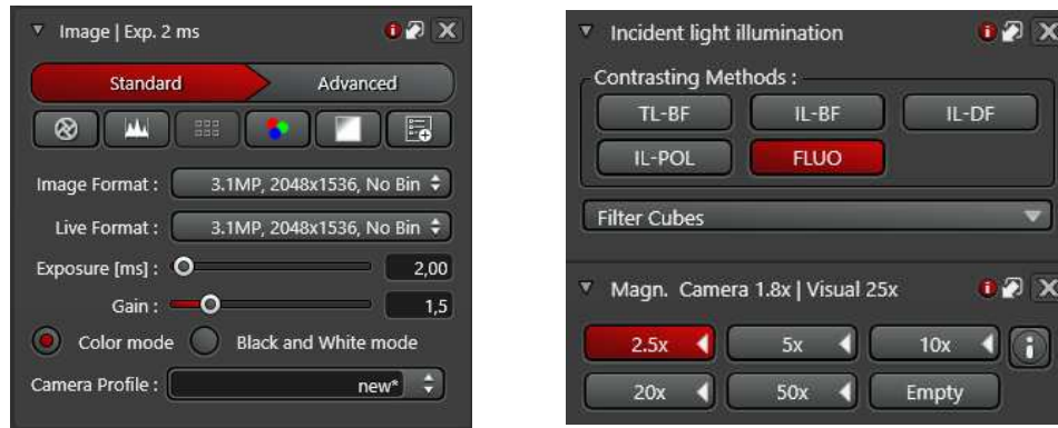
Figure 4-3 – Settings for fluorescent image capturing in LAS X
