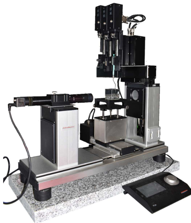
Figure 4-6 – Experimental Setup – Pendant Drop
