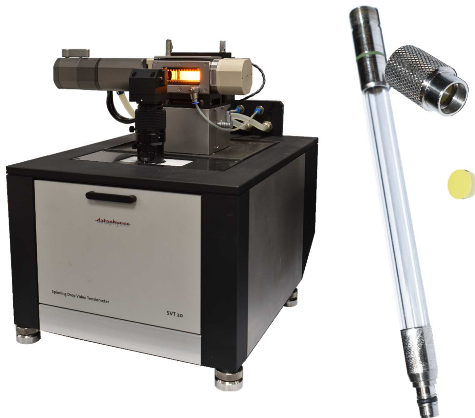
Figure 4-7 - - Experimental Setup – Spinning Drop
