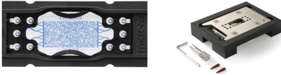
Figure 46 – The representation of the micromodel chip and the chip holder (Schnöpf, 2019).
