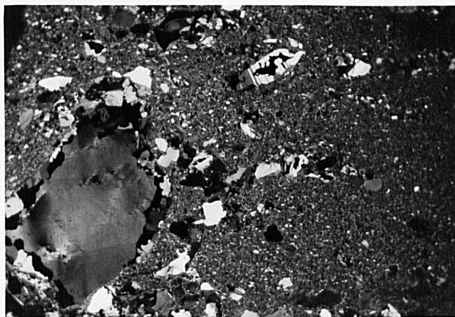
Fig. 4.20: Albite-galena paragenesis in siltstone, surrounding a detrital quartz grain. Base of picture = 5.6 mm (+).
