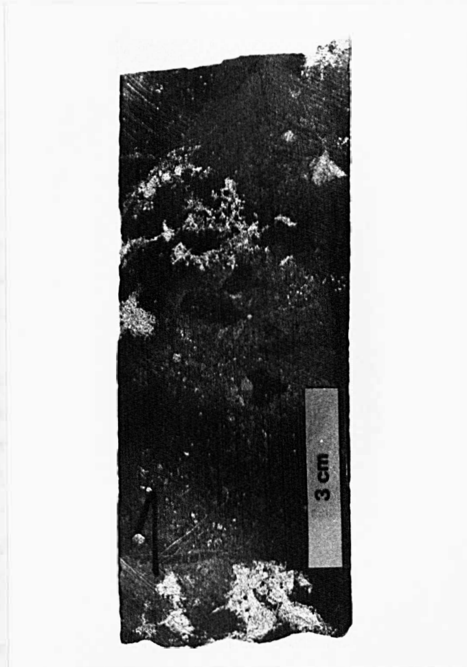
Fig. 3.05: Brecciation of chloritic siltstone in the stringer zone. The fine-grained matrix is mineralized (chalcopyrite).
