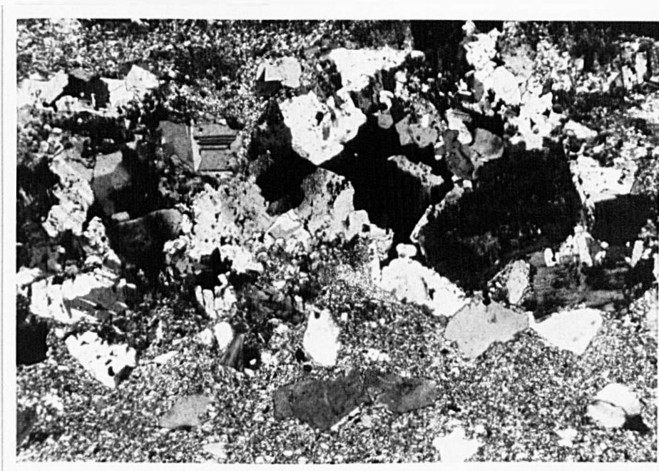
Fig. 4.02: Galena associated with albite and hyalophane. Base of picture = 3.6 mm (+).
