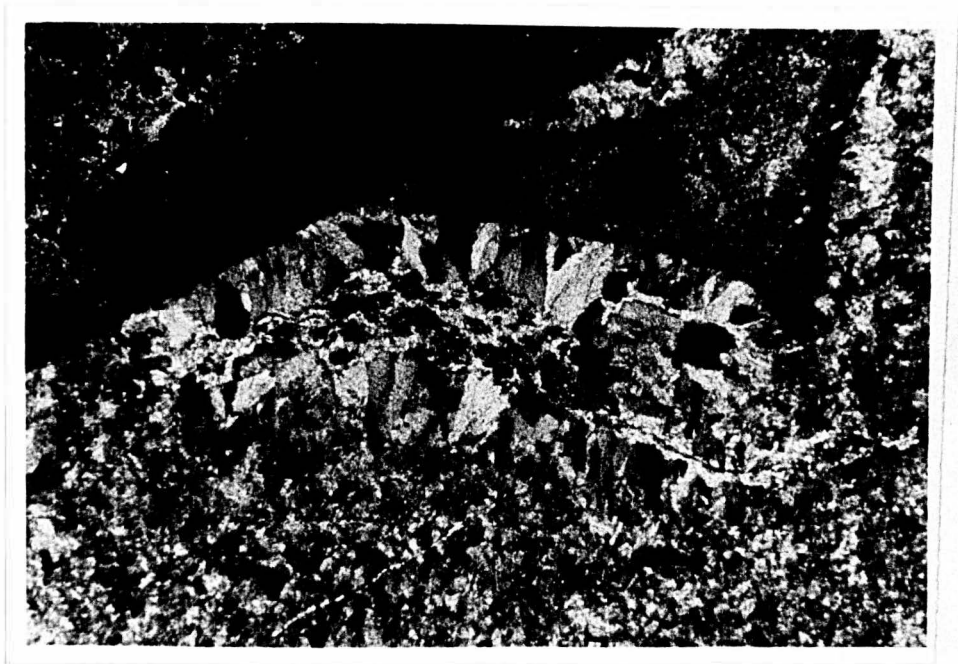
Fig. 3.28: Nodule in micrite. Acicular carbonate crystal along the margins and diffuse, cherty quartz in the centre. Base of picture = 3.6 mm (+).
