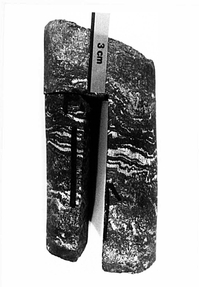
Fig. 4.25: Black zone type magnetite-carbonate laminae in core specimen from the 46 - 40 prospect.
