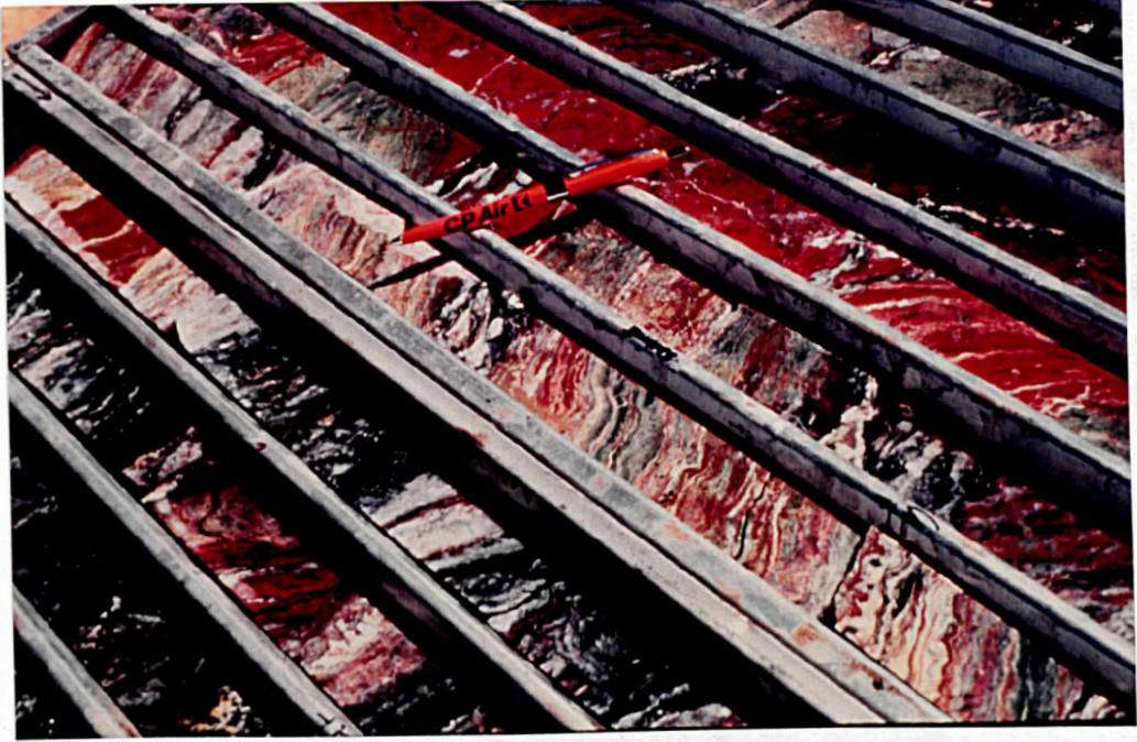
Fig. 3.23: Drill core from the red zone with layers of hematite, jaspilite, quartz, carbonate and magnetite.
