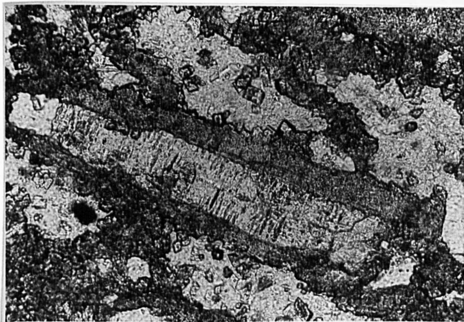
Fig. 3.36: Ca-carbonate plus quartz pseudomorph after gypsum, within ferroan dolomite and quartz. Base of picture = 0.9 mm (-).
