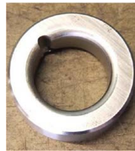
b) Ball valve seat damage (Langbauer, 2017)
