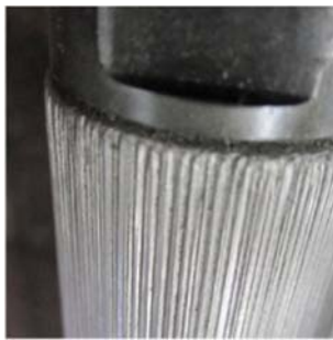
a) Plunger surface damage (Don-Nan, Ed., 2018)
