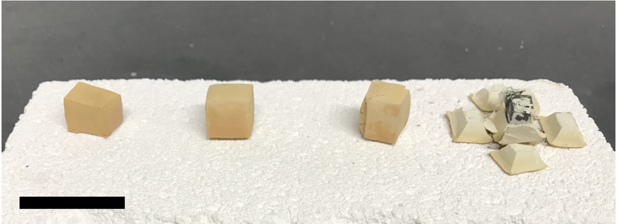
Figure 4.10: Samples after heat treatment for 23 h at 1300 °C in atmosphere. Increasing Zr content from left to right: Ti-46.5Al, Ti-46.5Al-2Zr, Ti-46.5Al-4Zr and Ti-46.5Al-8Zr. Convex surfaces of the cubes and cracks in the oxide scale are more pronounced the higher the Zr content of the sample. Scale bar length is 2 cm.
