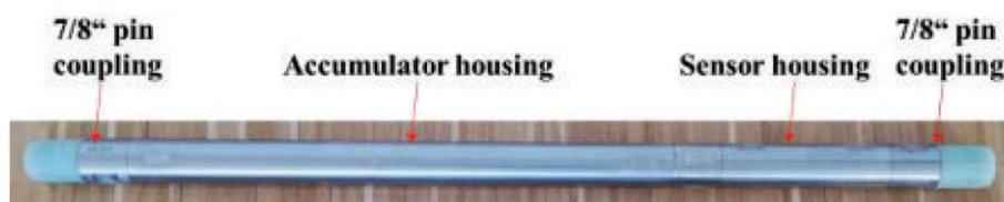
Figure 22: Downhole dynamometer sensor (DDS) (Langbauer et al., 2019)
