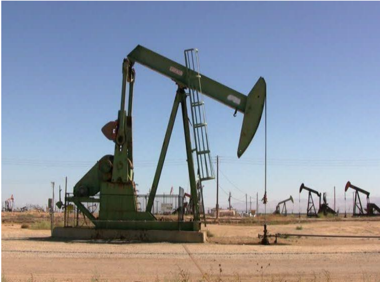
Figure 1: Picture of a sucker rod pumping system (Aurelio, 2019)
