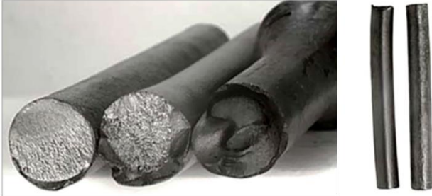
Figure 7: Bent rod failures (Norris, 2007)
