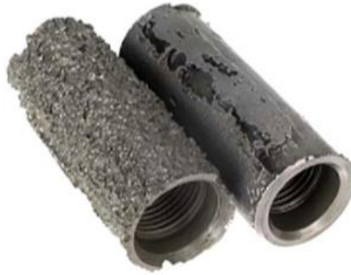
Figure 9: CO 2 corrosion on couplings (Norris, 2007)
