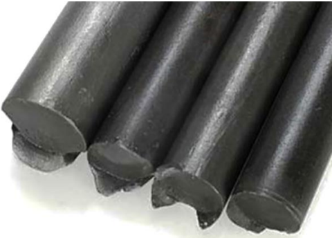
Figure 8: Surface damage failures (Norris, 2007)
