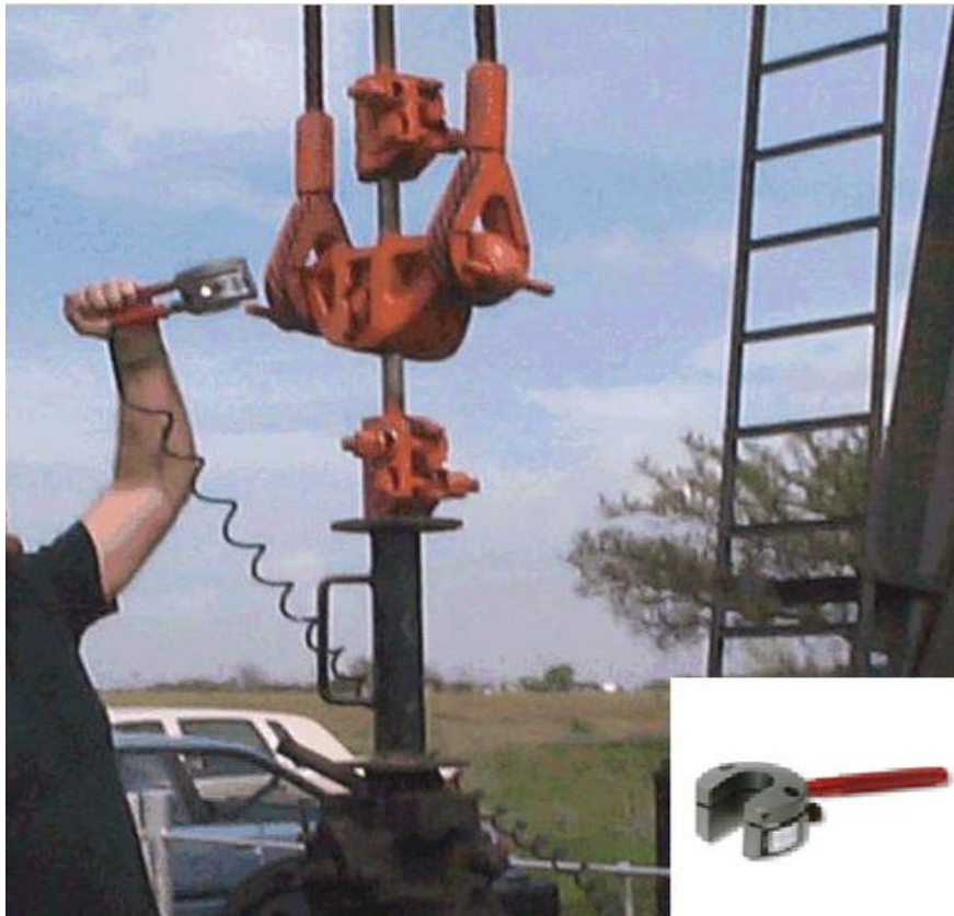
Figure 13: Installation of a horseshoe dynamometer (Downhole Diagnostic, 2020)
