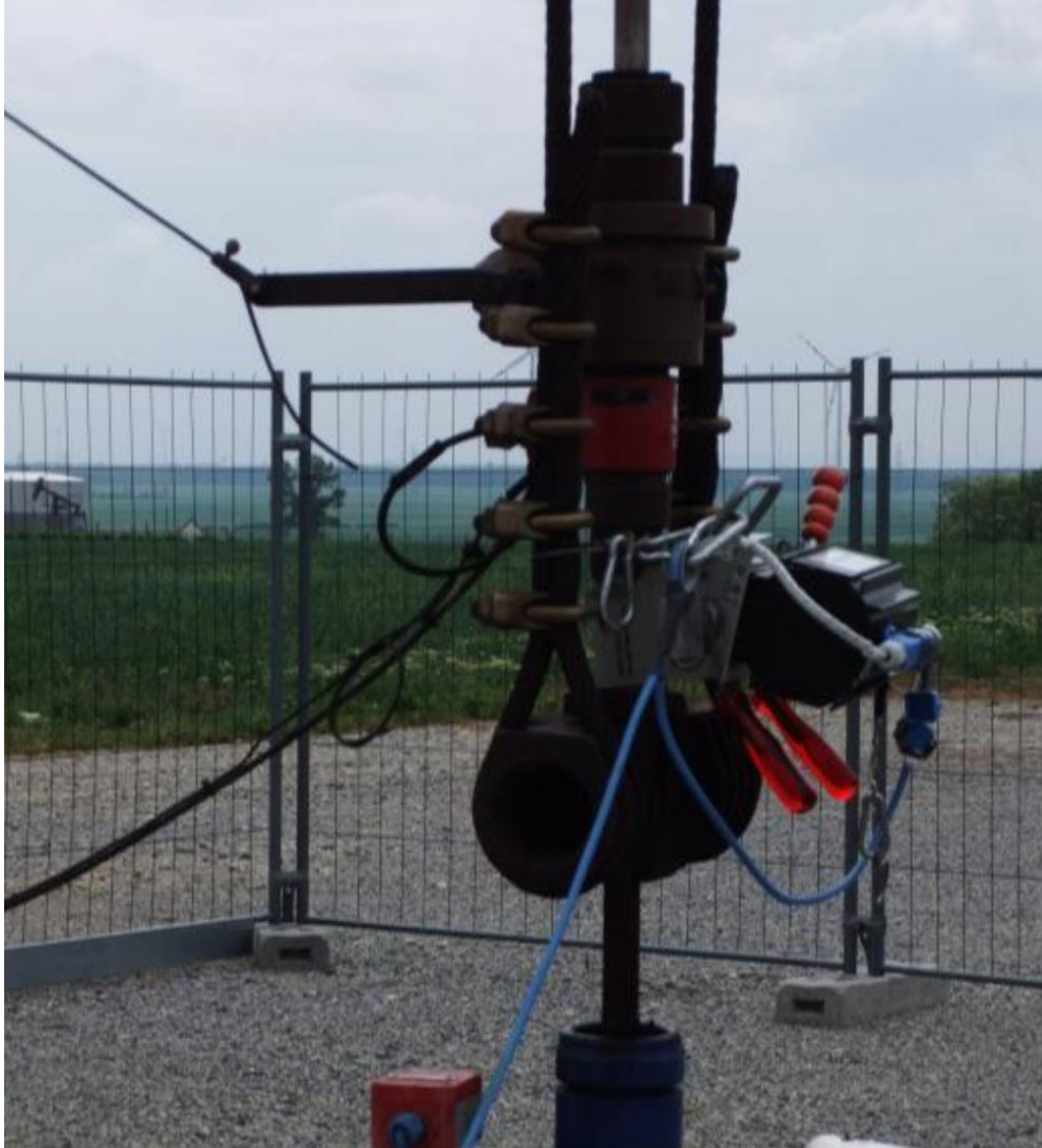
Figure 12: Electrical downhole dynamometer (Langbauer, 2019)
