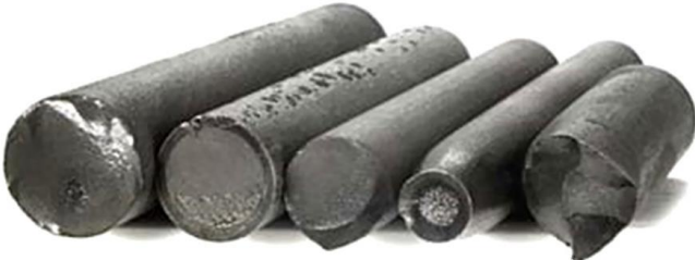
Figure 5: Tensile or fatigue failures (Norris, 2007)
