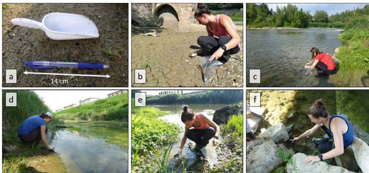
Figure 7 (a) Plastic shovel used for the sampling campaign. Examples of sampling with the plastic shovel at sample sites (b) PE11, (c) ARNVIII, (d) US15, (e) ARNXII and (f) CI5.
