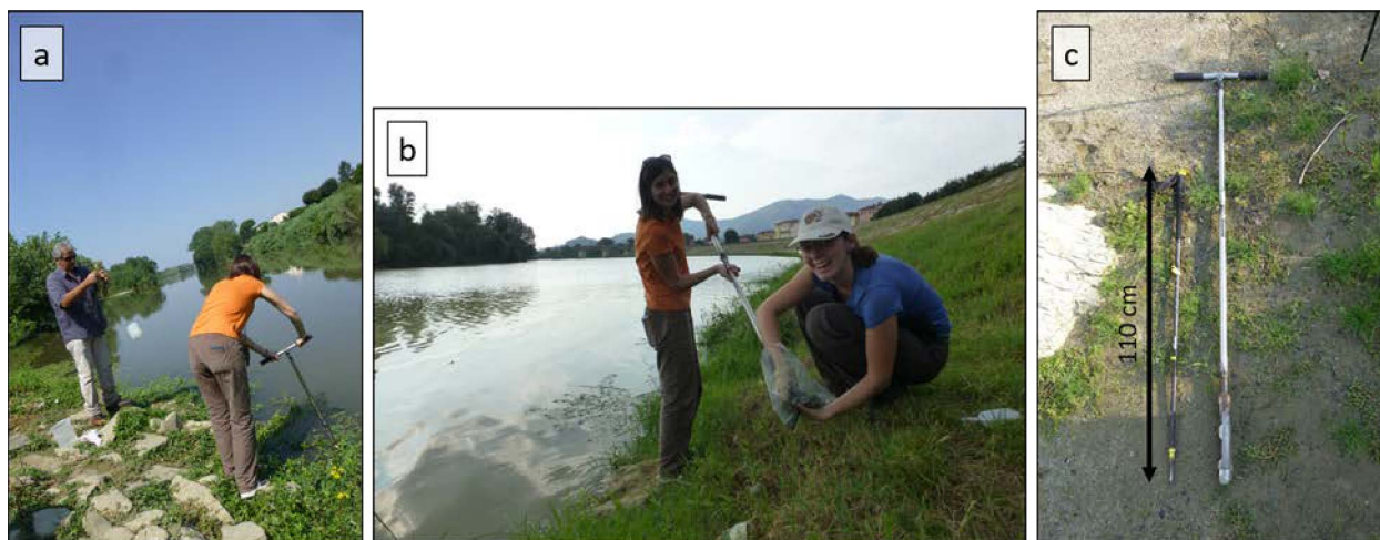
Figure 6 Collection of stream sediments in shallow water areas using a stainless steel hollow-core sampler here illustrated at sample sites (a) ARNXIII and (b) ARNXV. (c) Stainless steel hollow-core sampler.
