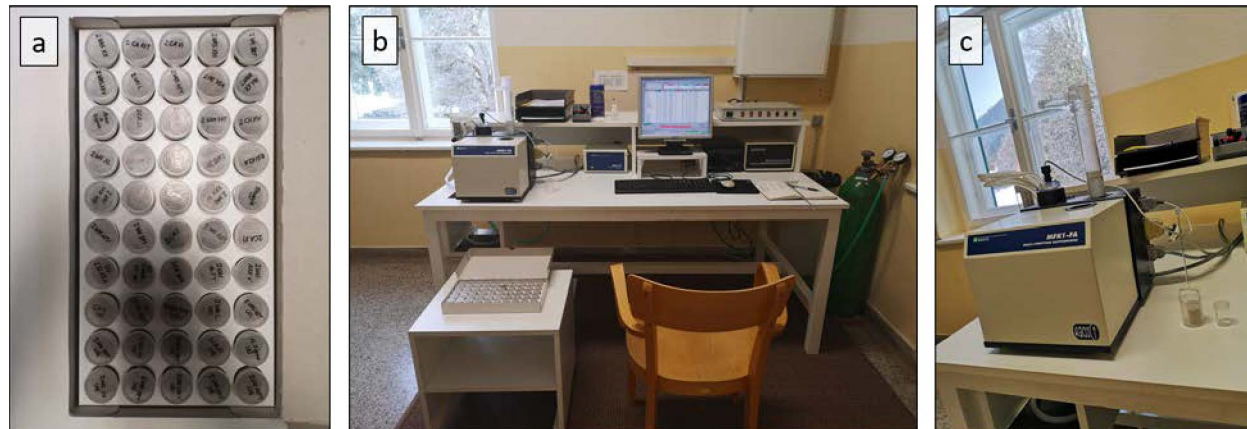
Figure 8 (a) Powder Samples in plastic cylinders; (b) and (c) setup for measuring the magnetic susceptibility with an AGICO MFK1.
