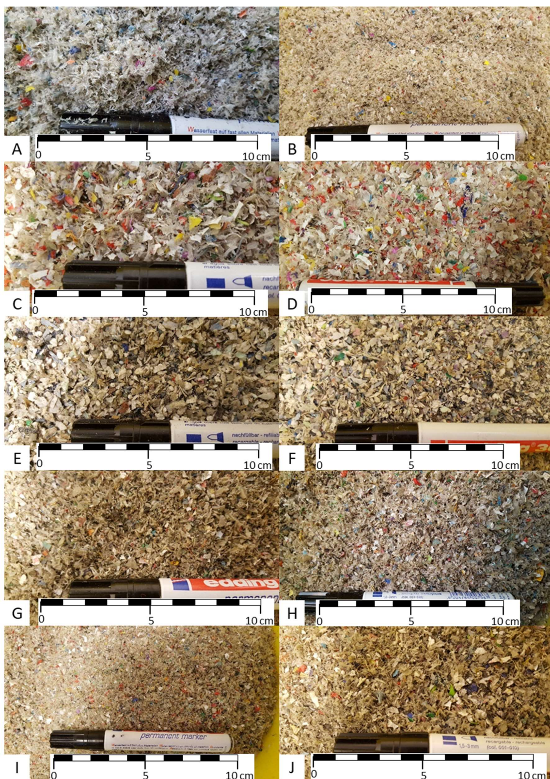
Figure 14. Exemplary photos of the flakes of all investigated materials after shredding to < 4 mm: P_PE—A; P_W,PE—B; P_PP—C; P_W,PP—D; P_PS—E; P_W,PS—F; PO_A—G; PO_W,A—H; PO_B—I; and P—J.
