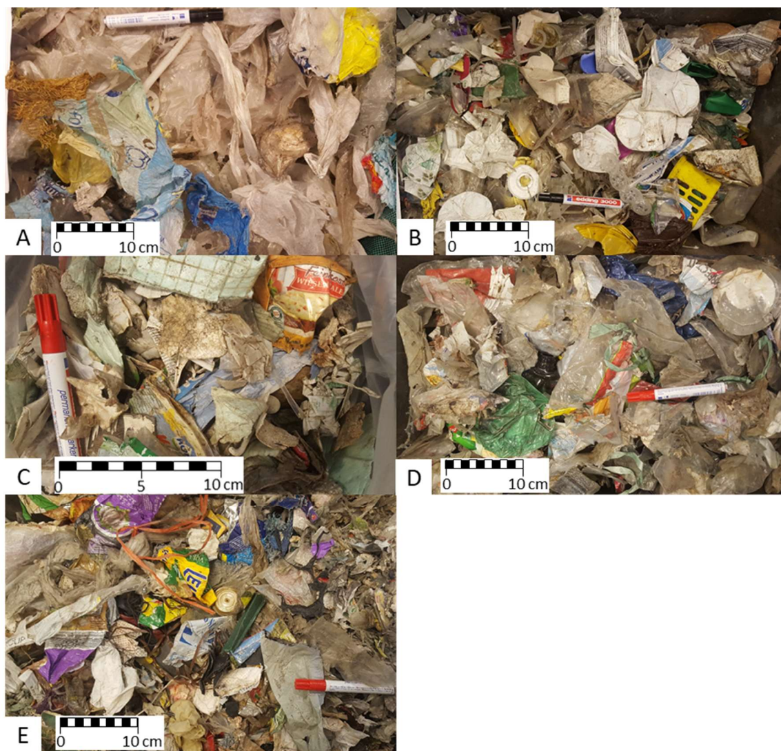
Figure I3: Exemplary photos of plastic types sorted with NIR: PE—A; PP—B; PET—C; PS—D; and others—E.
