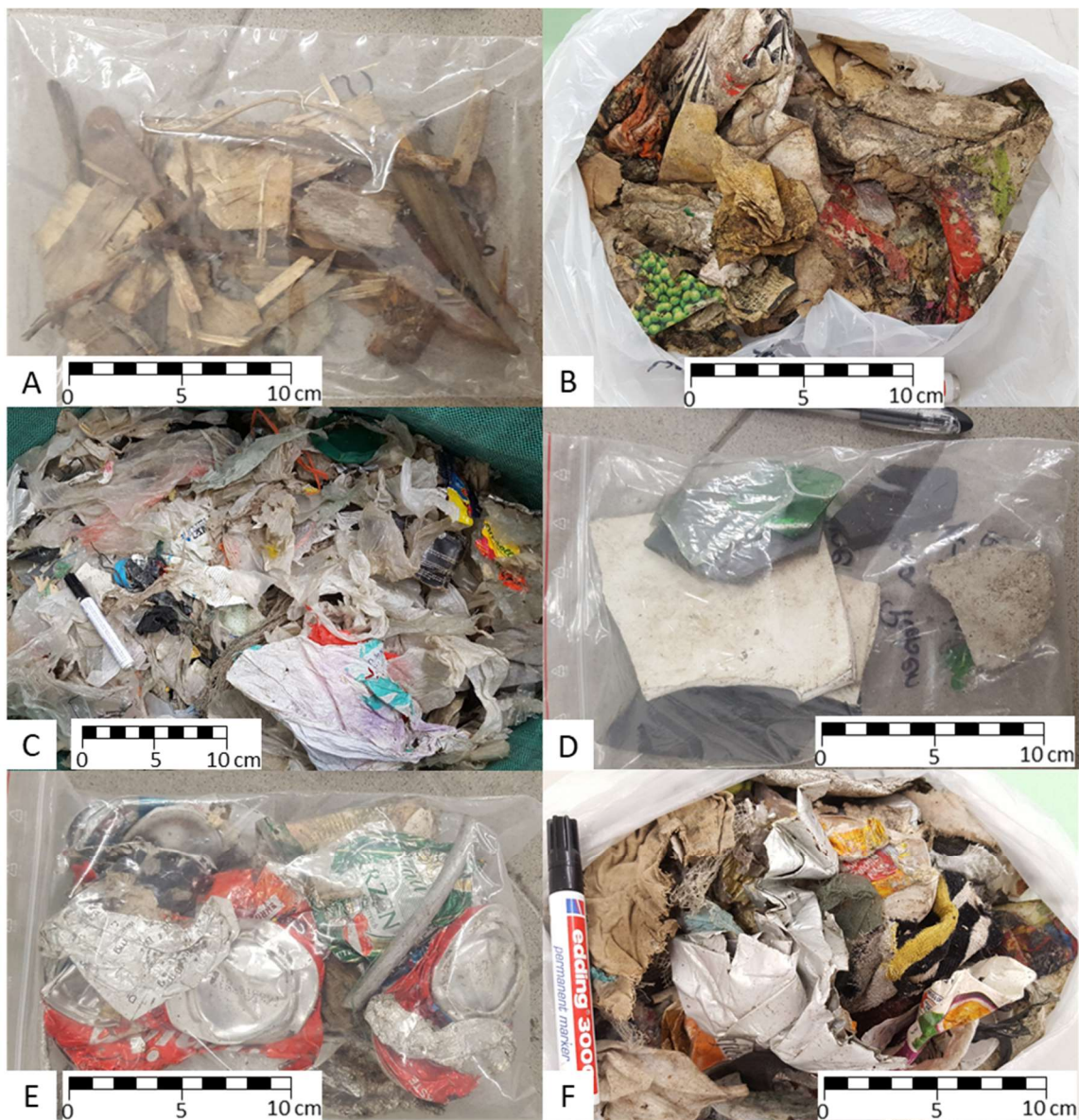
Figure 12. Exemplary photos of the manually sorted material fractions: wood—A; P&C—B; plastics—C; inert—D; metals—E; others—F.
