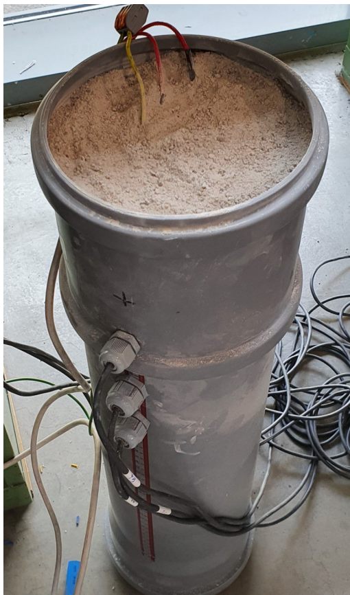
(a) Filling process of the Thermo-Pipe.
