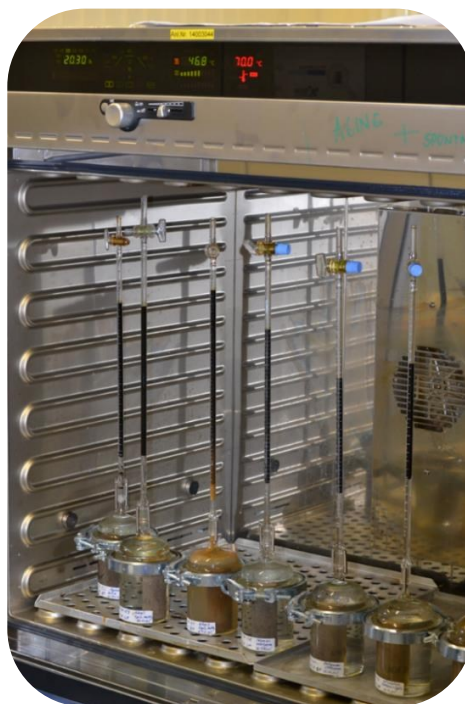
Figure 1 – Aging of Cores under Reservoir Temperature in the Oven (Arekhov, 2019)
