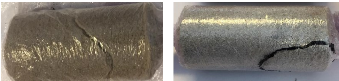
Figure 3.1 Sandstones probes (labelled as code B16390 – right and B16407 – left). Both are unconsolidated sandstones
