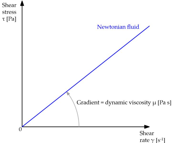
**Figure 7: Rheology diagram for a Newtonian fluid (derived from Caenn et al. 2017)**
