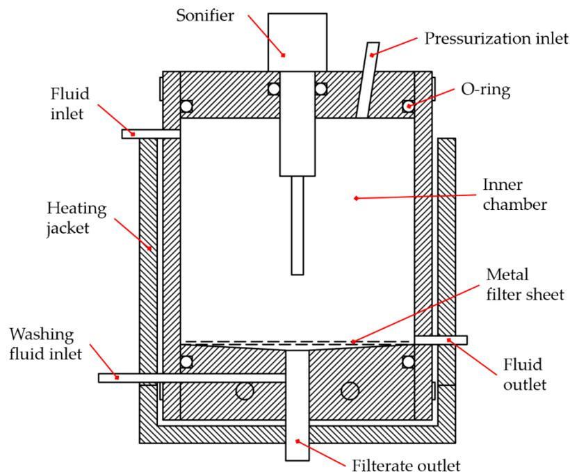
**Figure 36: Schematic of the automated fluid loss cell (derived from Tehrani and Cameron 2008)**
