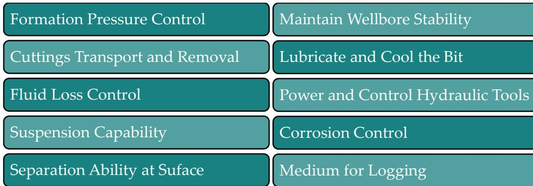
**Figure 3: Overview of drilling fluid functions (derived from Caenn et al. 2017)**
