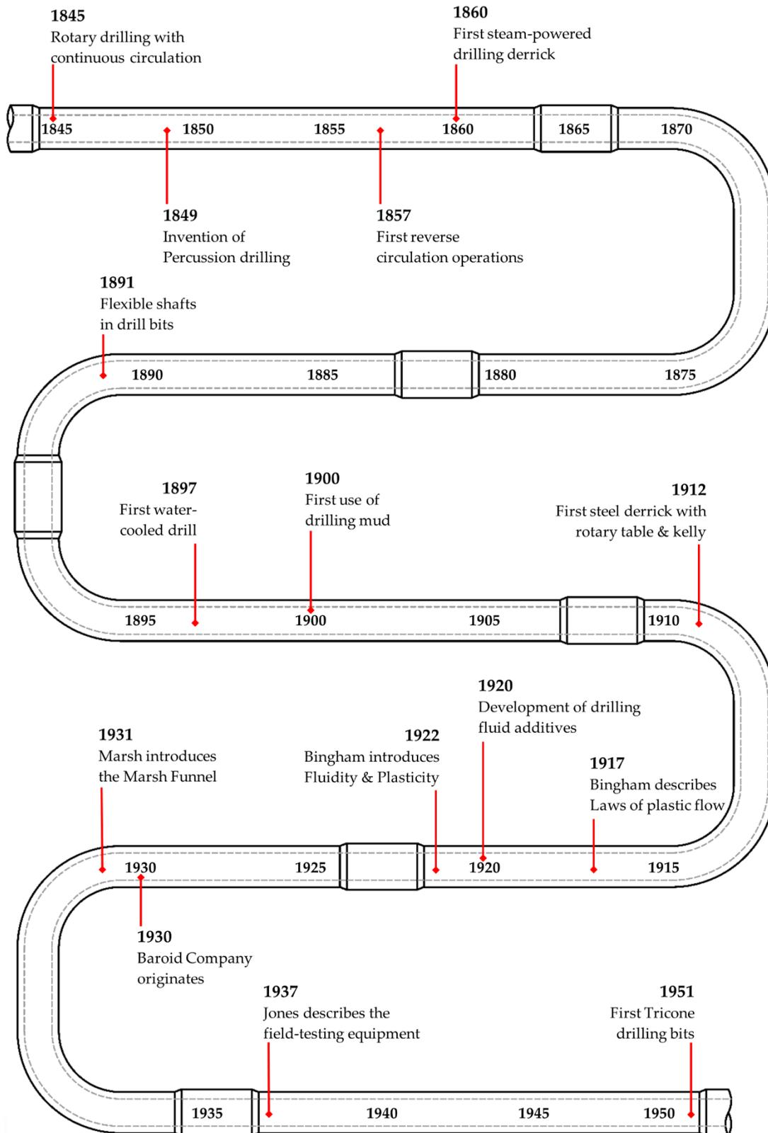
Figure 1: Historical overview of drilling fluids from 1845 – 1950
