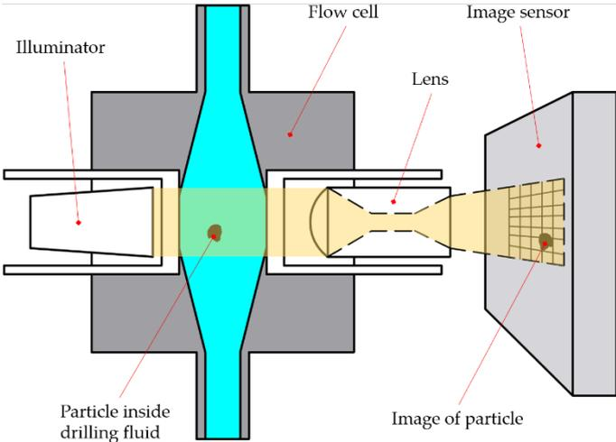
**Figure 37: Schematic of automated liquid particle analyzer (derived from J.M. Canty 2020b)**
