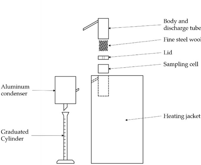
**Figure 19: Exploded view schematic of a 10 milliliters retort (derived from Fann Instrument Company 2020g)**
