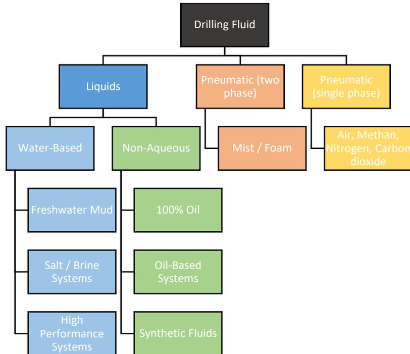
**Figure 6: Overview of drilling fluid systems (derived from ASME 2011; Caenn et al. 2017)**
