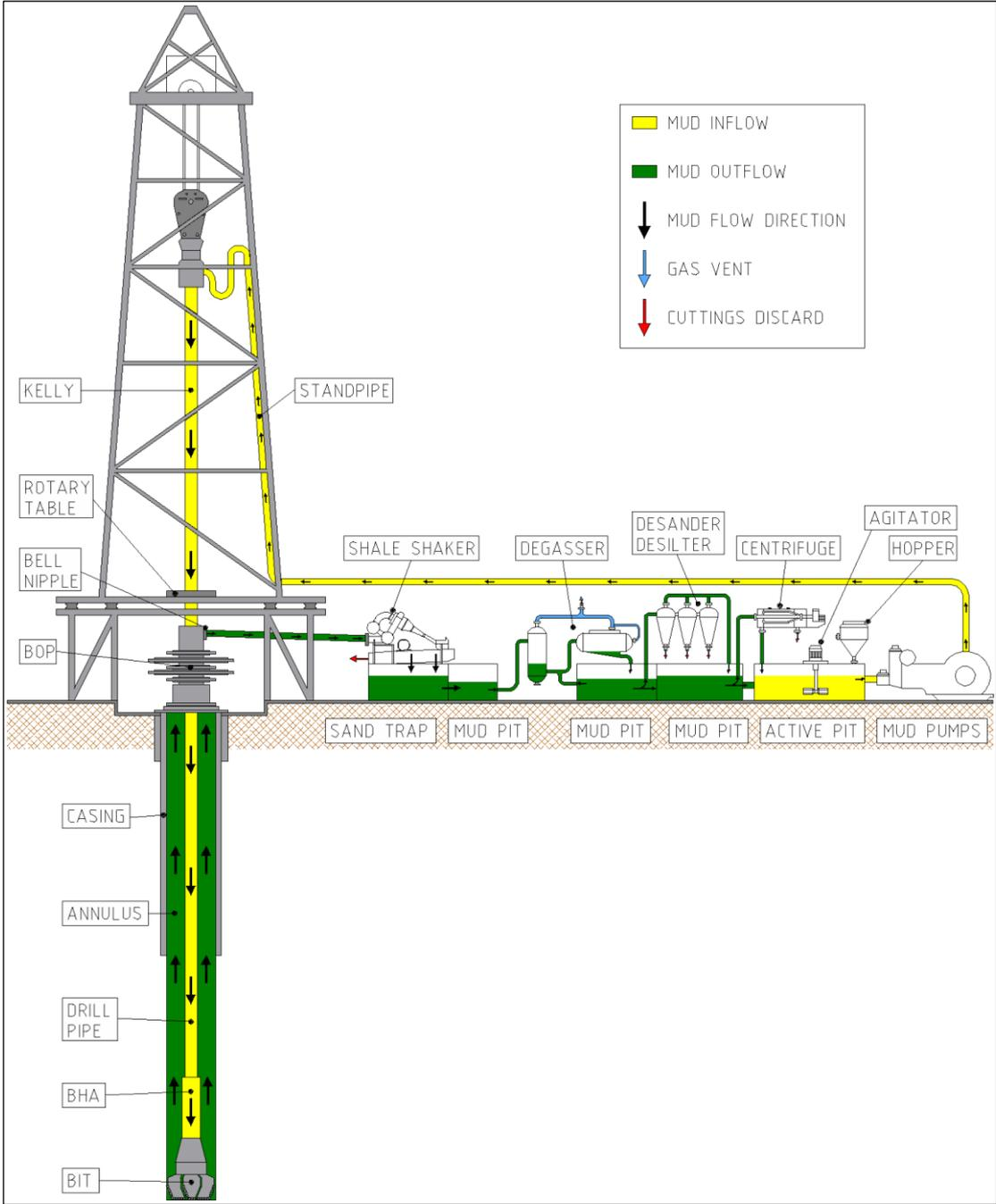
Figure 11: Drilling Fluid Circulation System
