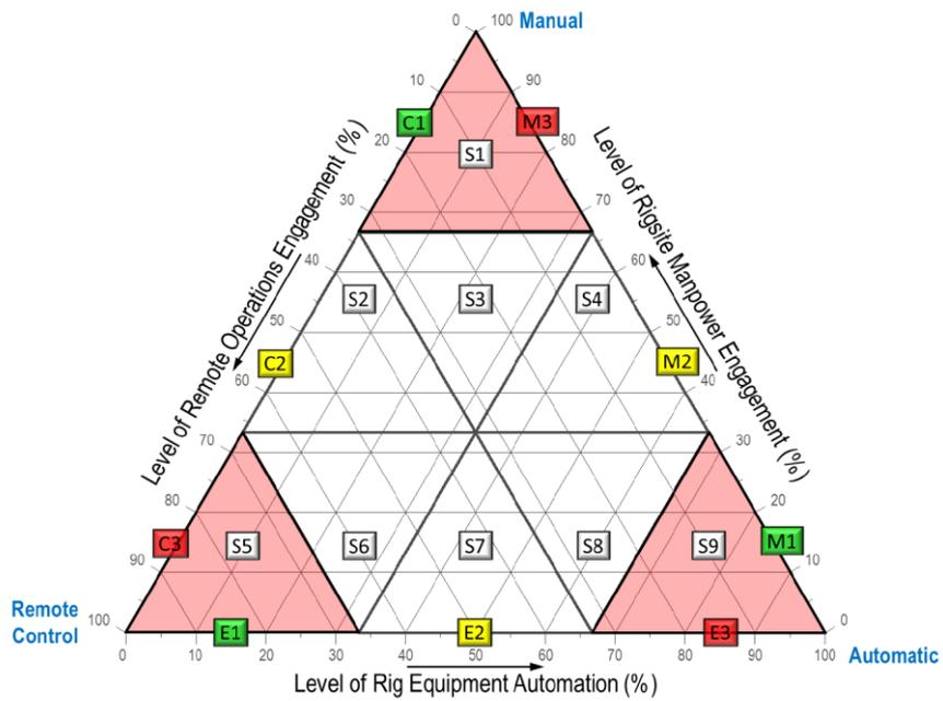
Figure 26: Drilling systems automation ternary chart subdivided into nine taxonomy segments and nine binary segments. (Zamora and Hildebrand 2013)
