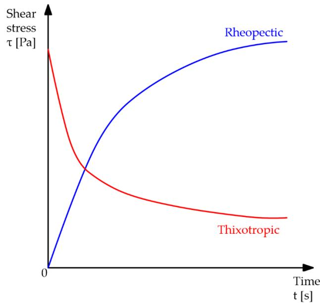
**Figure 9: Shear stress versus time diagram for thixotropic and rheopectic fluids (derived from Monicard 1982)**
