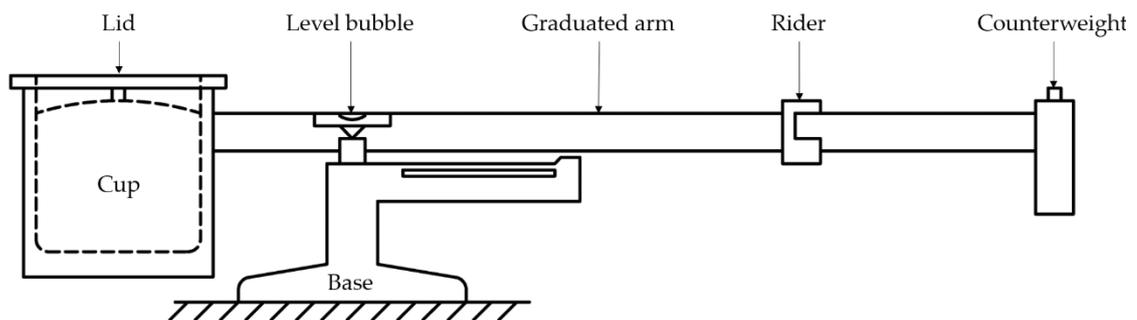
**Figure 16: Schematic of a mud balance**
