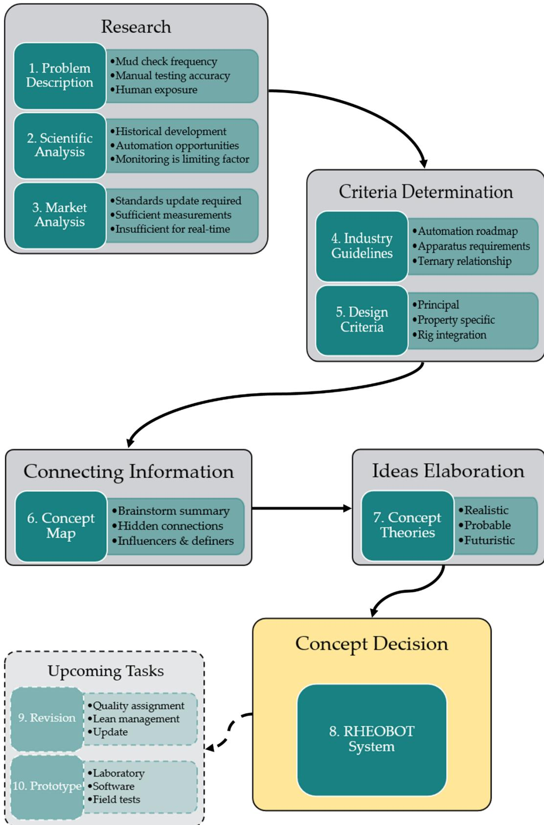
Figure 23: Overview of the conceptual design process
