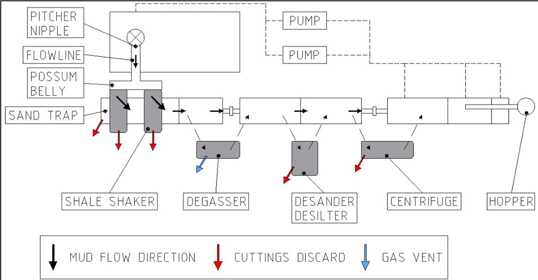
Figure 13: Layout of typical solids control equipment (derived from Philips 2011)
