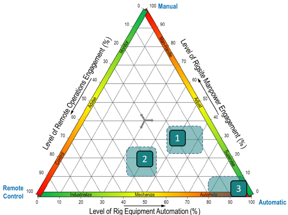
**Figure 31: Position of the three concept ideas in the ternary design chart. (adapted from Zamora and Hildebrand 2013)**
