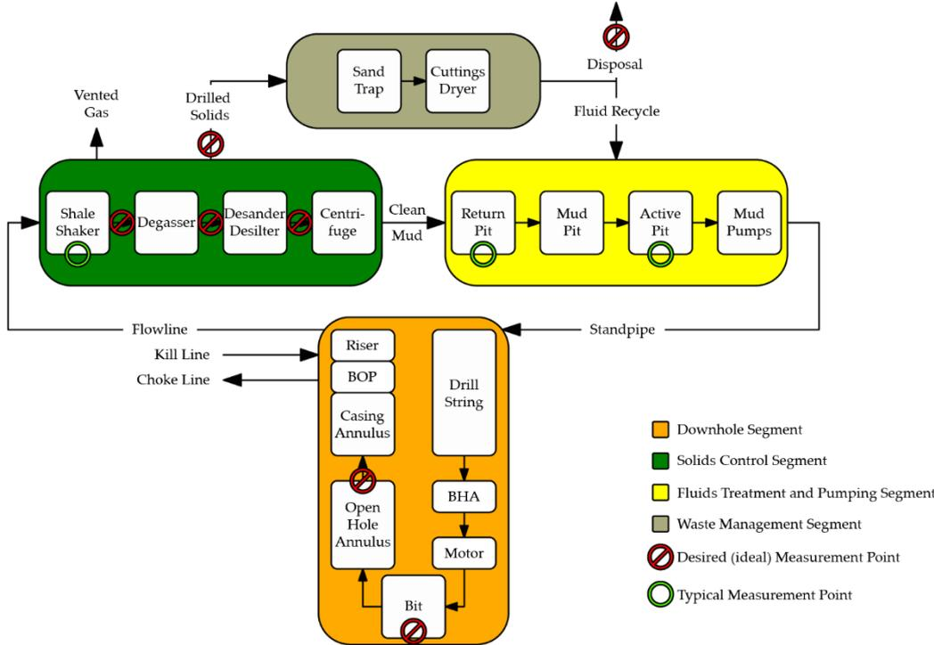
Figure 14: Drilling fluids system with typical and desired measurement points (derived from Geehan and Zamora 2010)
