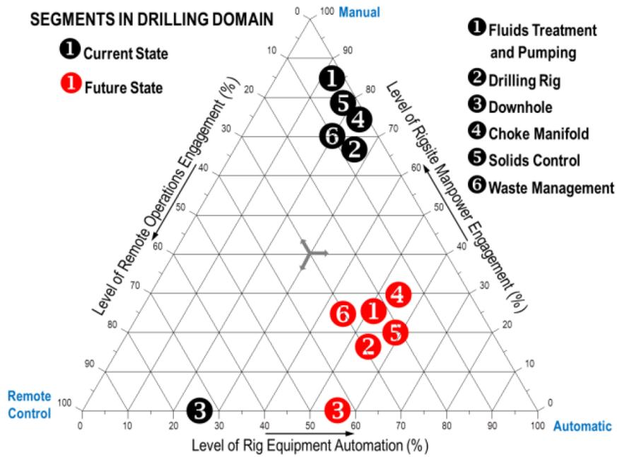
Figure 27: Current and Future States for the six drilling domain segments. (Zamora and Geehan 2013)
