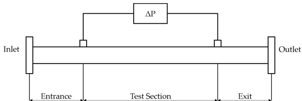
**Figure 34: Schematic of pipe rheometer principle (derived from Taugbøl et al. 2019)**
