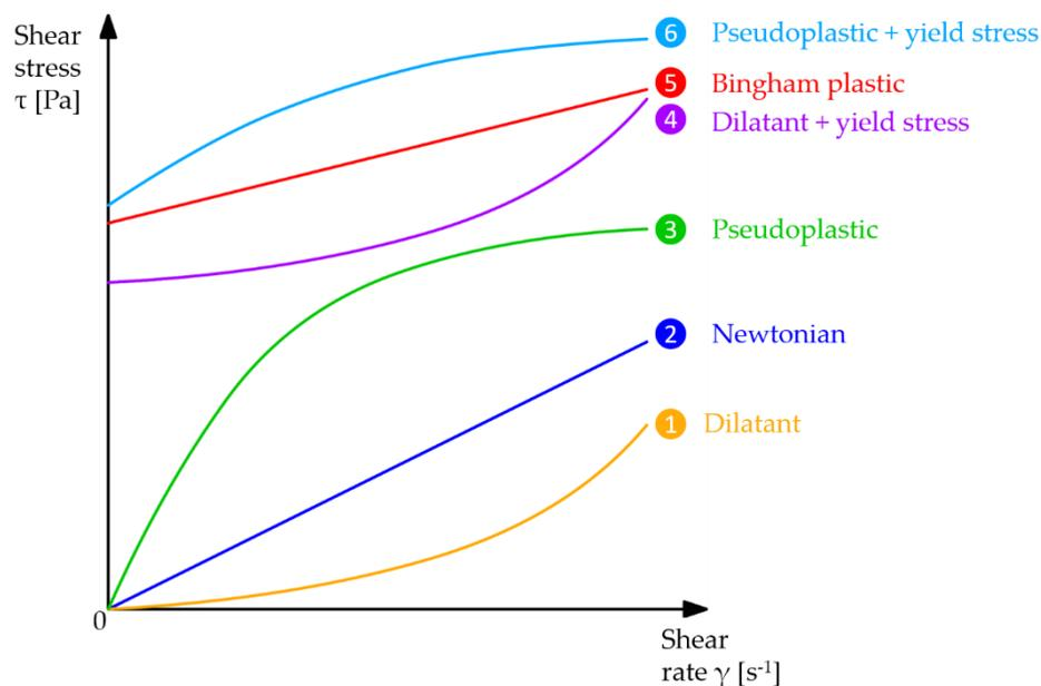
**Figure 8: Rheogram for different types of rheological fluid behavior (derived from Sikorski 2002; Caenn et al. 2017)**
