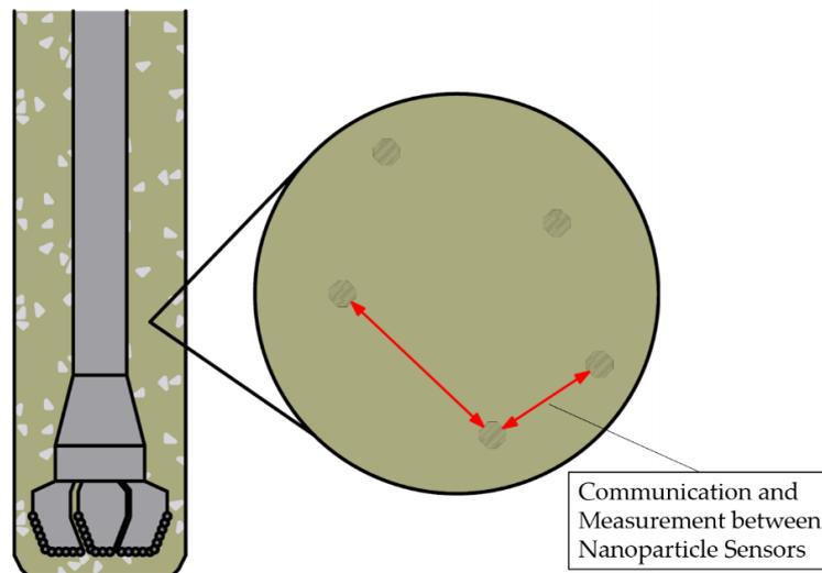
**Figure 32: Graphical illustration of nanoparticle sensors for third RHEOBOT idea**
