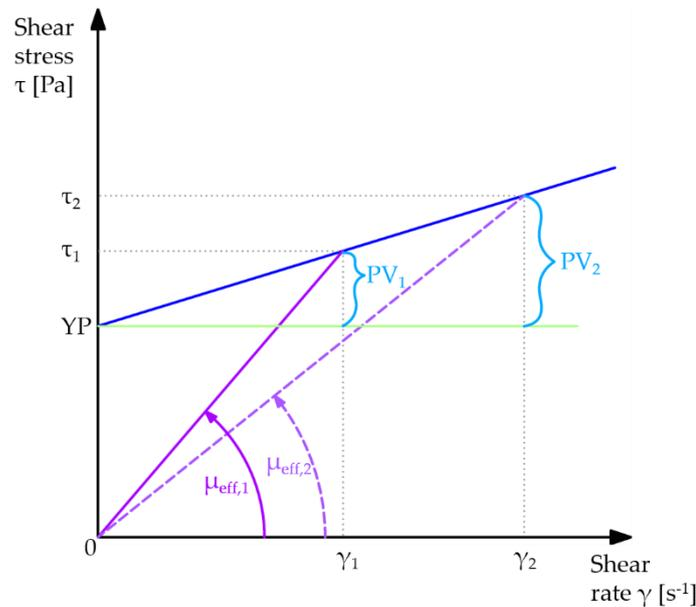
**Figure 10: Rheological diagram for a Bingham plastic model (derived from Caenn et al. 2017)**
