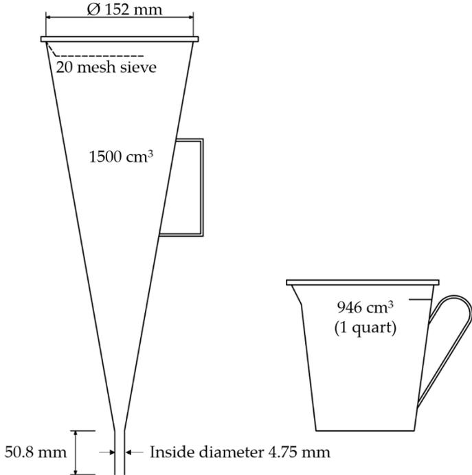
Figure 17: Schematic of a Marsh funnel and viscosity cup (derived from Marsh 1931)
