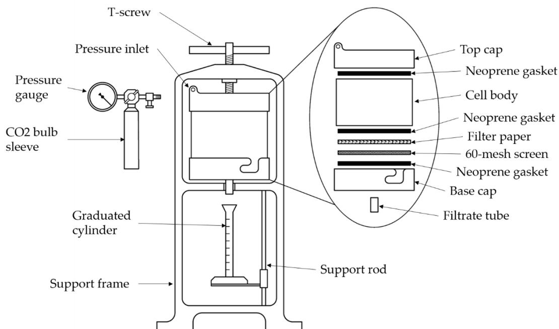
**Figure 20: Schematic of a filter press with detail of test cell**
