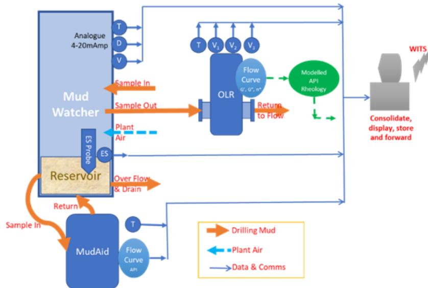
**Figure 22: Setup of the OFI Automated System (Kamal et al., 2020)**
