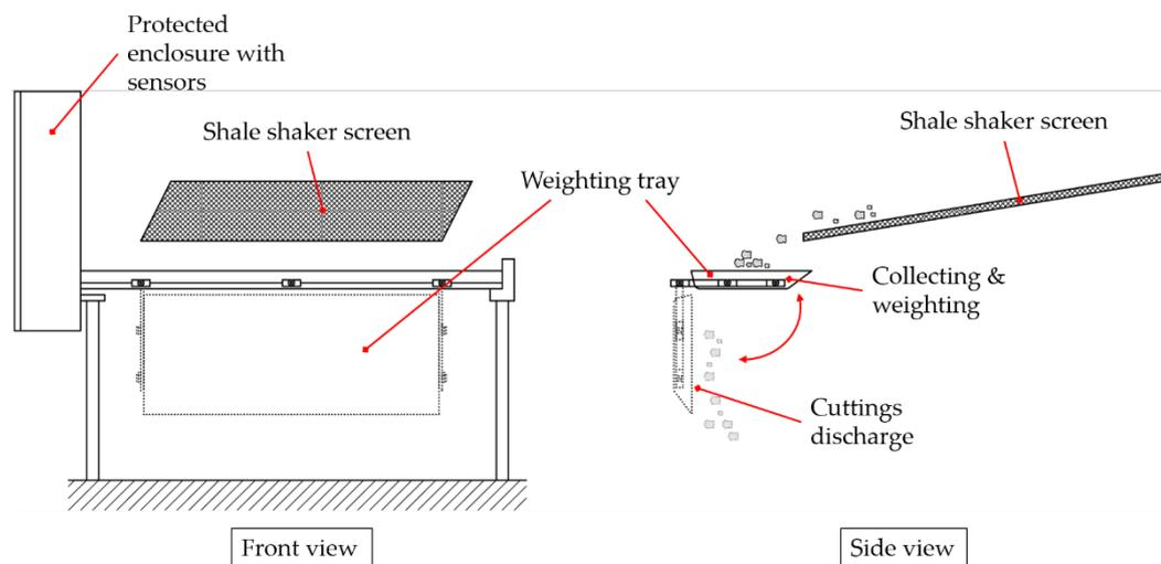
**Figure 38: Schematic of Cuttings Flow Meter (derived from Naegel et al. 1998)**
