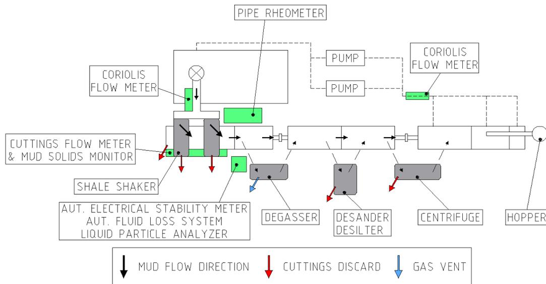
**Figure 40: Integration of the components of the first RHEOBOT concept idea**
