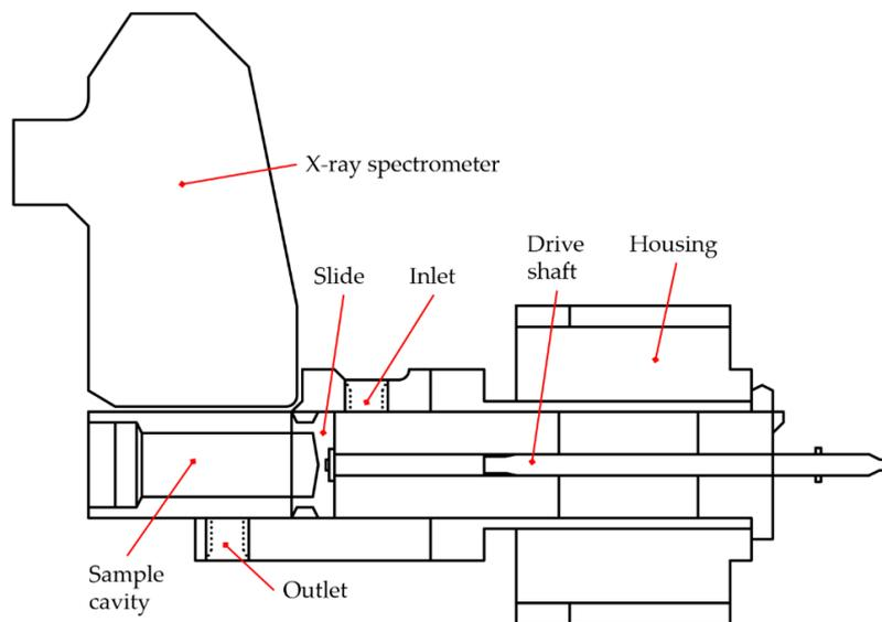
**Figure 39: Schematic of Mud Solids Monitor test chamber (derived from Stock et al. 2013)**
