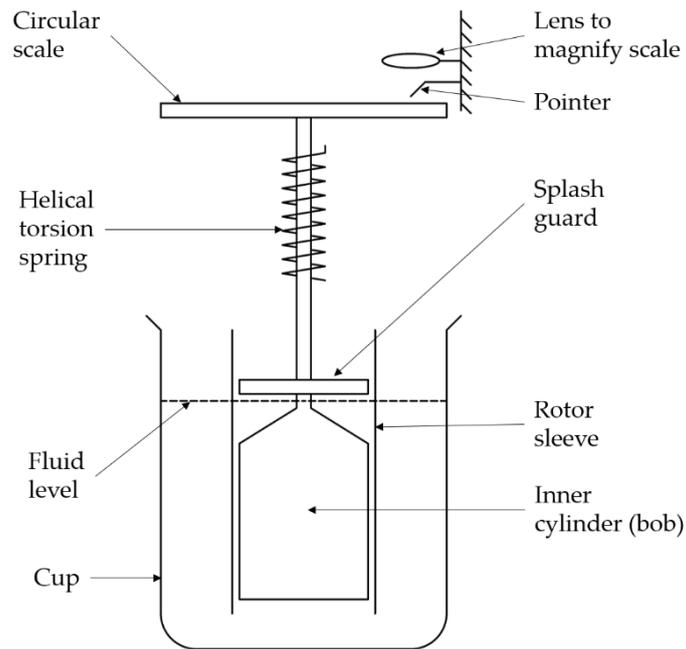
**Figure 18: Schematic of a rotational viscometer (derived from Lam and Jefferis 2014)**
