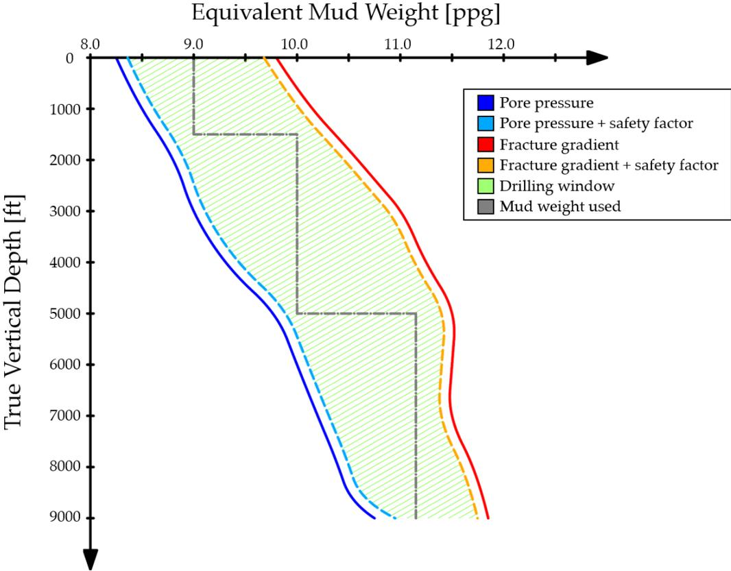
Figure 4: Example of a mud weight window
