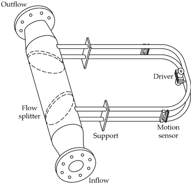
**Figure 33: Schematic of Coriolis flowmeter (derived from Anklin et al. 2006)**
