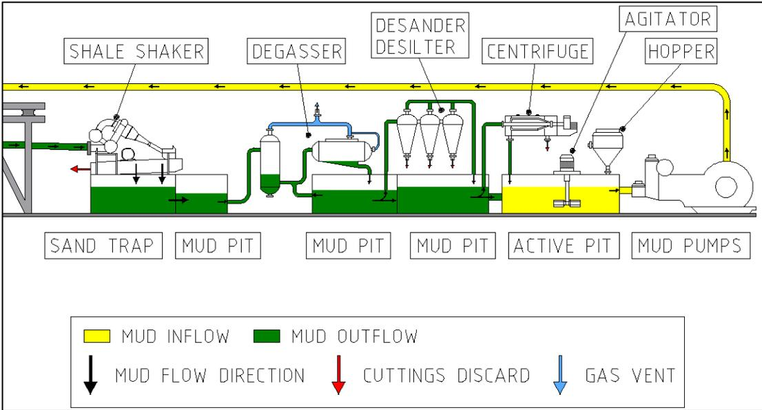
Figure 12: Sectional view of typical solids control equipment
