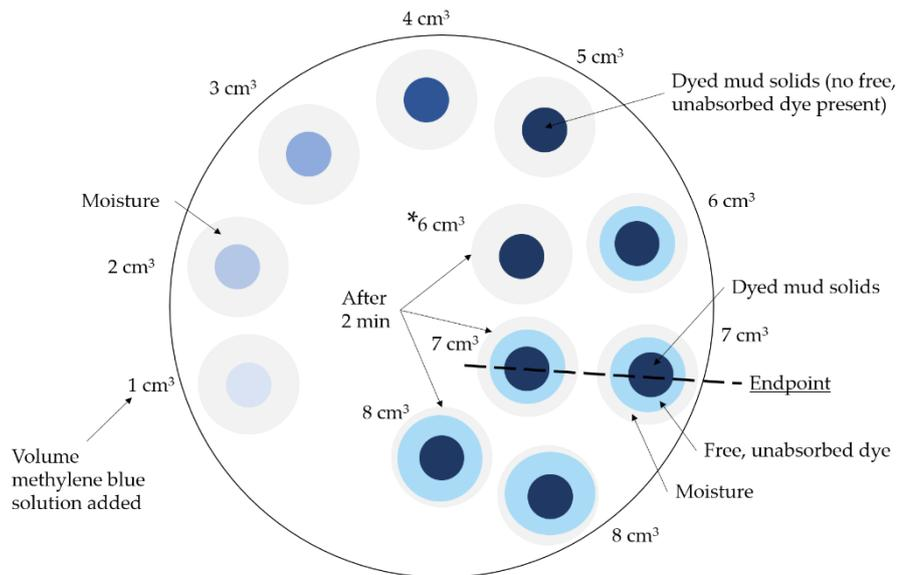
**Figure 21: Spot test for the endpoint of the methylene blue titration test. (\*After two minutes the filter paper absorbs the free dye detected immediately after adding the sixth cm<sup>3</sup> and indicates that the endpoint has not quite been reached.)**
