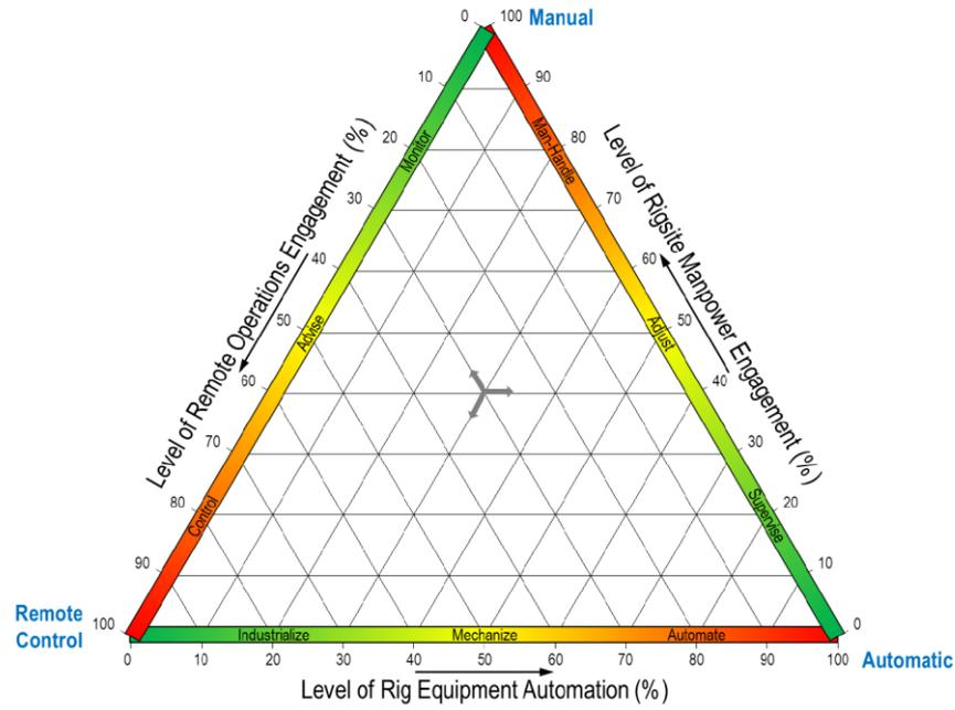
Figure 25: Framework for drilling systems automation ternary design chart. (Zamora and Hildebrand 2013)
