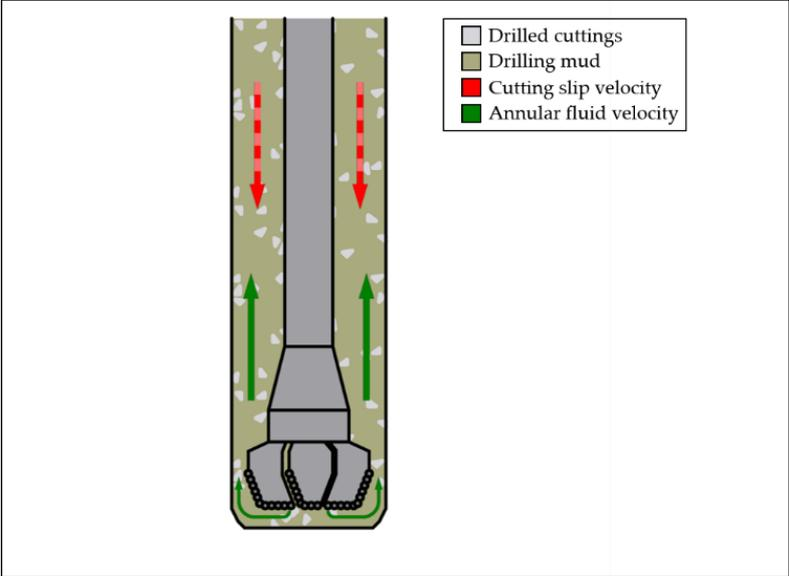
**Figure 5: Schematic of a wellbore with the drill bit. The figure shows the annular and the cutting slip velocity.**
