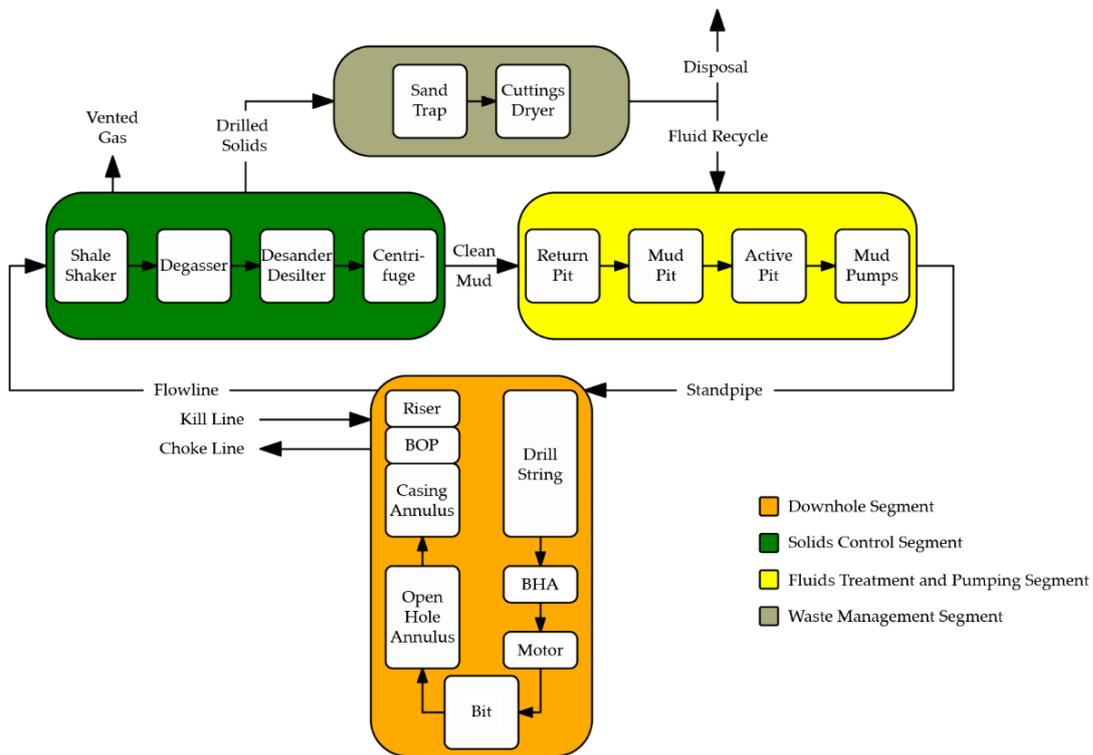
**Figure 29: Drilling fluids system with the four categories and the associated equipment inside the individual drilling fluid segments. (derived from Geehan and Zamora 2010)**
