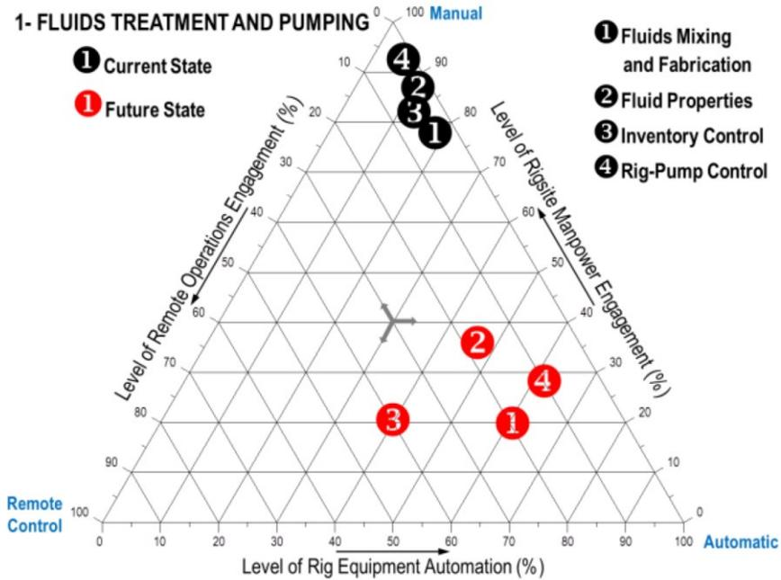
Figure 28: Current and Future States for fluids treatment and pumping systems. (Zamora and Geehan 2013)
