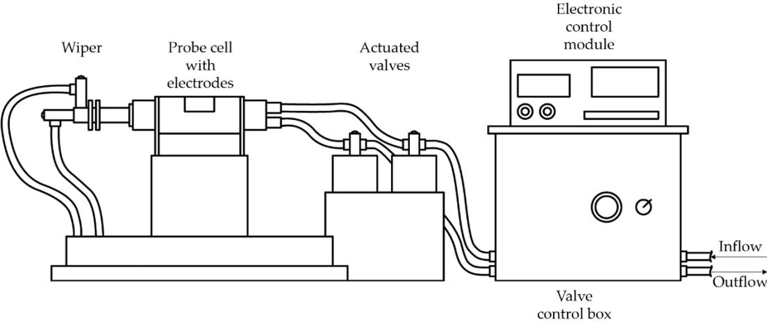
**Figure 35: Schematic of automated electrical stability meter (derived from Growcock et al. 2007)**
