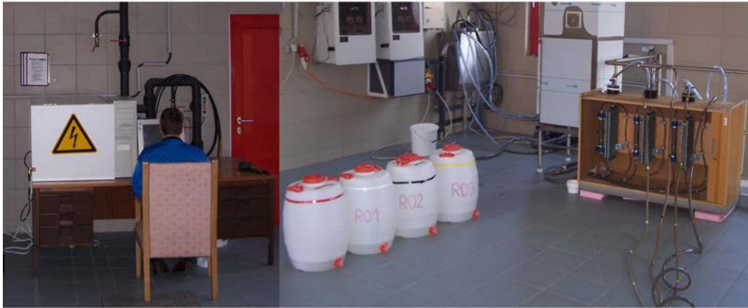
Fig. 2: Tech scale unit; left side: controlling station, right side: reactor unit
