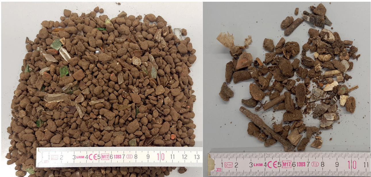
FIGURE 4: Reject (left) and eject (right) from SBS trial, water content 15 wt%, fraction 10-4.5 mm.
