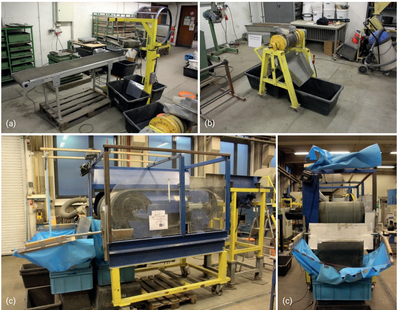
FIGURE 3: a) Overband magnetic, b) drum magnetic and c) Eddy-current separators.
