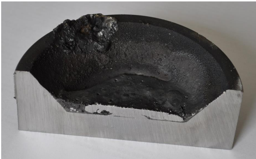
Figure 3-10: Cross-section of the crucible for Ex. 3.
