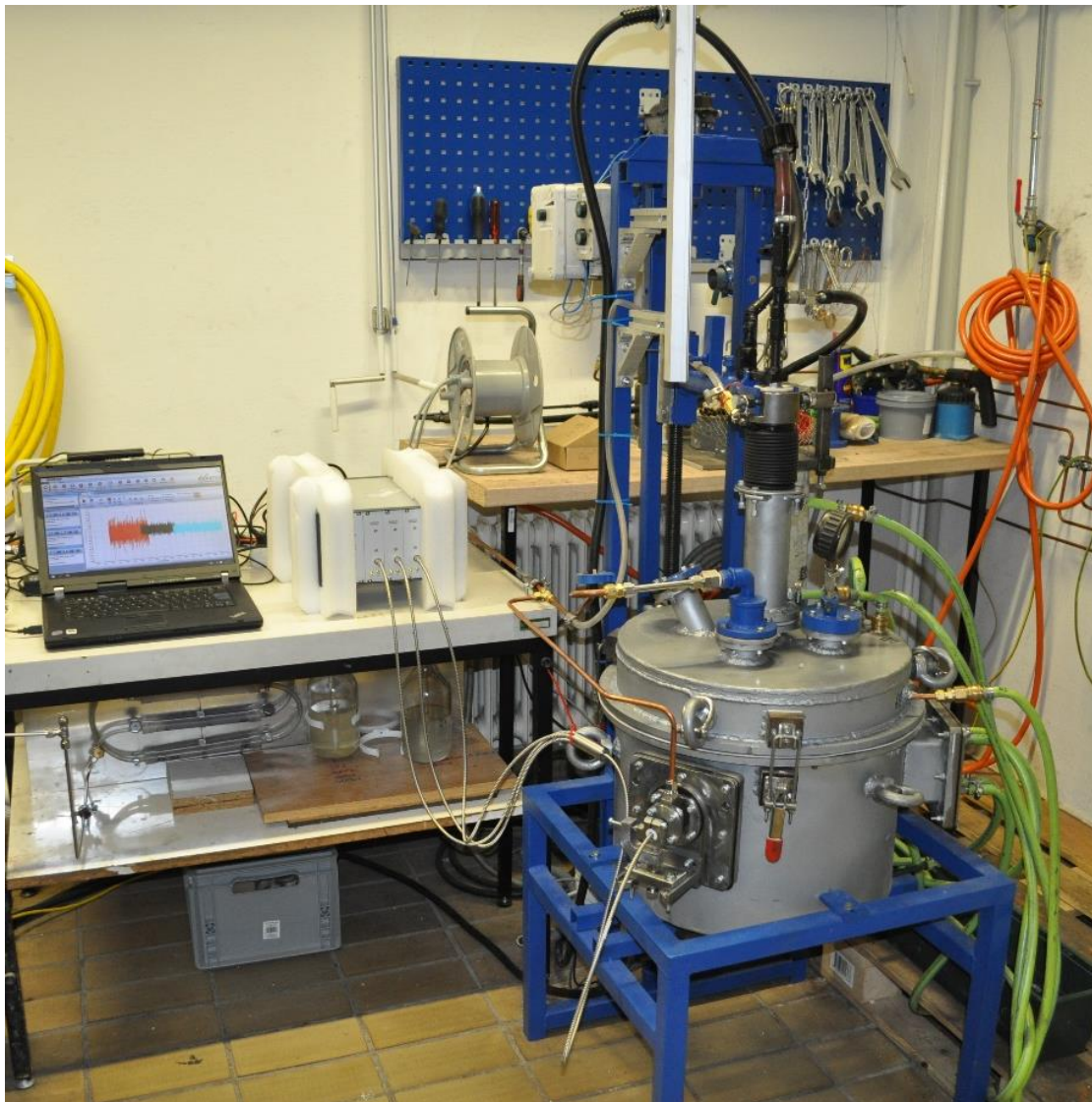
Figure 3-3: Setup of the plasma arc monitoring experiment
