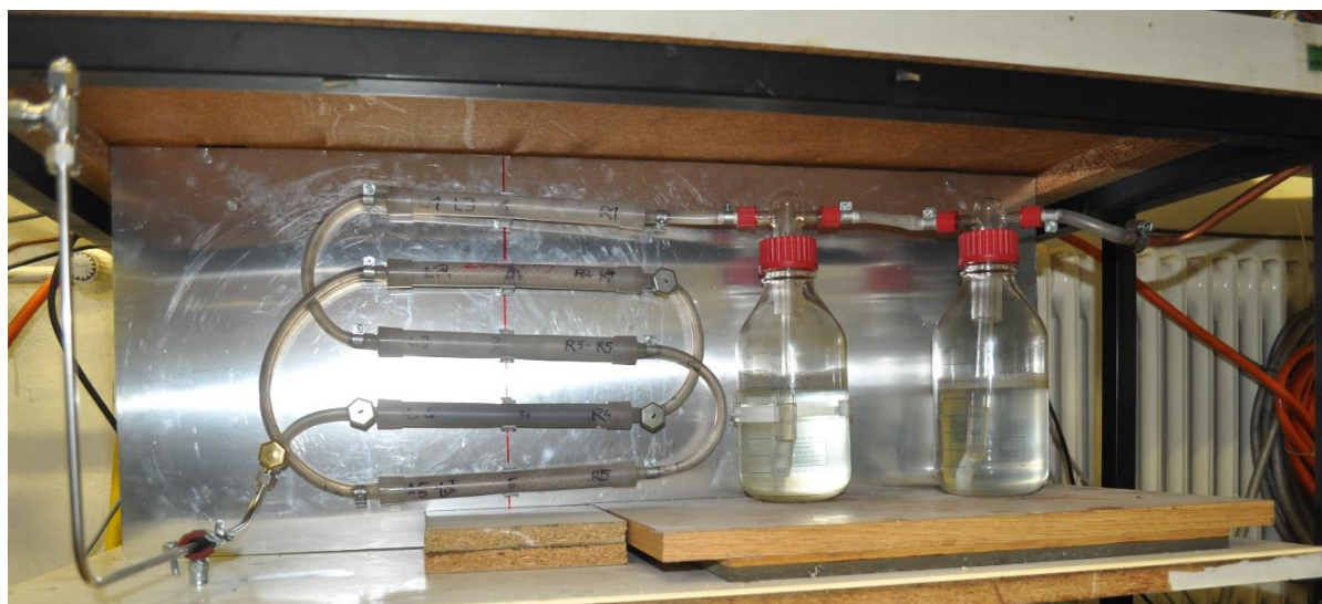
Figure 3-2: Setup of the off-gas cleaning system
