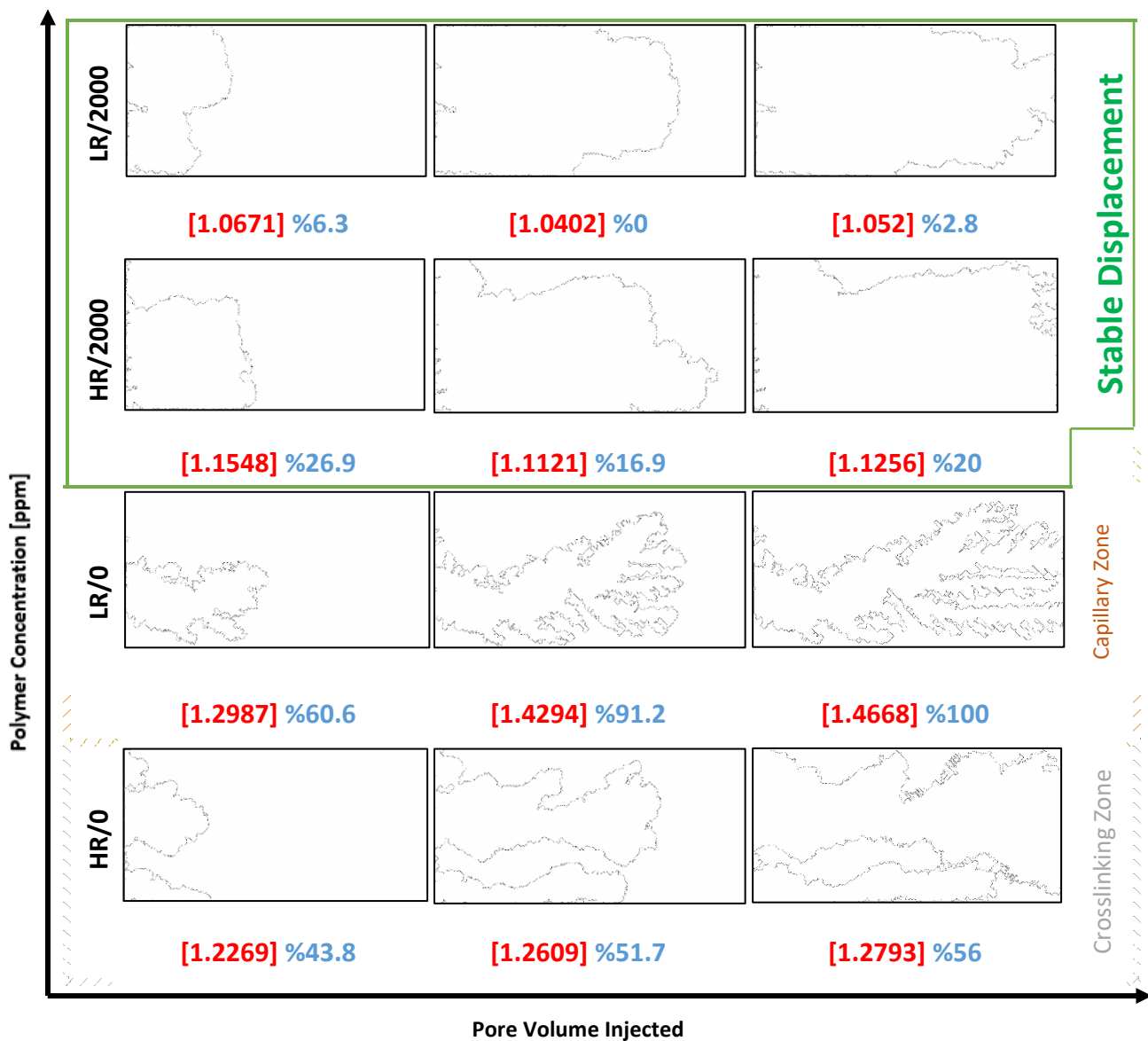
Figure 56: Sequence images of the displacement patterns and flow regimes as a function of polymer concentration and injected pore volume. The viscosity ratio ( M\mu ) is 2.9, 2.13 and 0.003 for the LR/2000, HR/2000 and waterflood scenarios, respectively. Red values in bracket are front fractal dimension while the blue percentages are their place in provided instability range, [1.0402-1.4668] so that the numbers are better felt.
