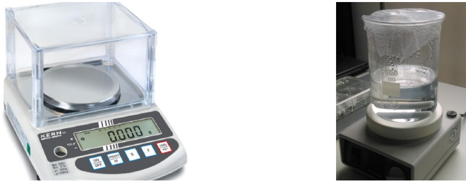
Figure 22. Left) Precision Balance and right) Magnetic stirring instrument with a beaker, containing the prepared solution.
