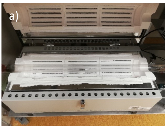
Figure 11.: a) Annealing furnace with the quartz boat inside the quartz tube, and b) Phase diagram of TiO 2 – temperature against pressure. [55]
