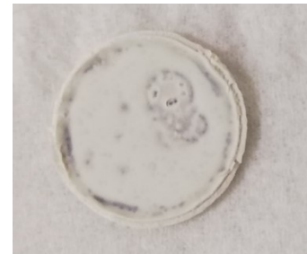
Figure 7.: Sample after thermal oxidation in air at 550 °C for 22 h
