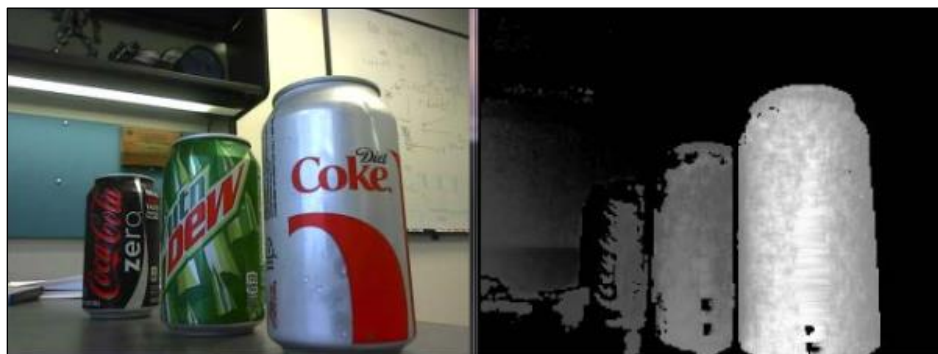
Figure 29: Input Image (Left) and a Depth Map (Right) (Li 2014)
