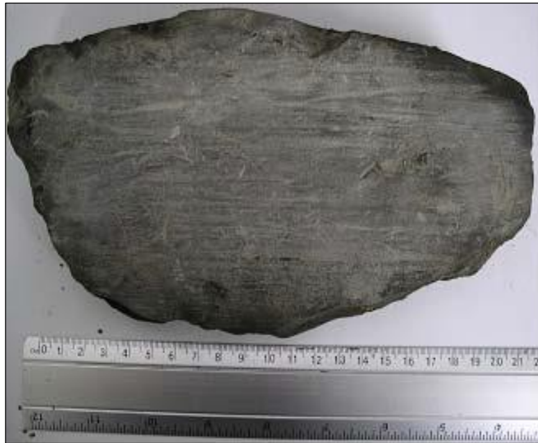
Figure 7: Large Tabular Caving Formed as a Result of Failure Along the Bedding Plane (Gallant, et al. 2007)
