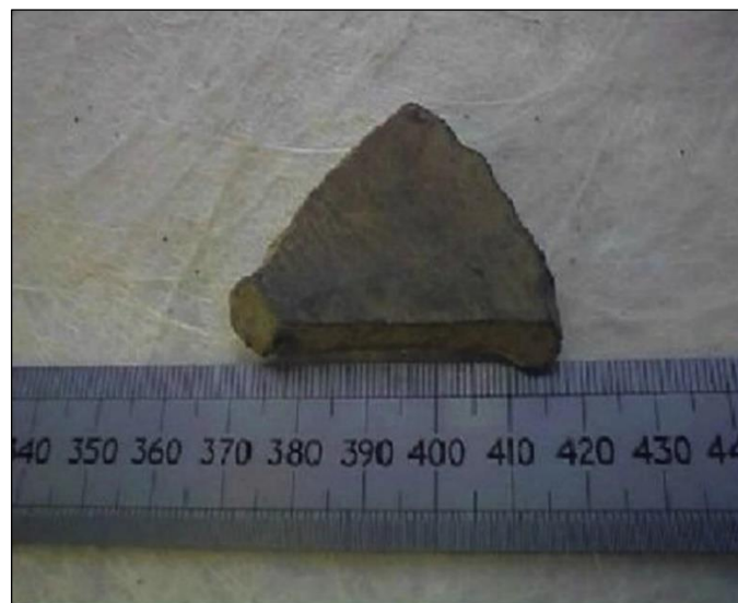
Figure 6: Example of a Tabular Caving. The Flat Surface of Bedding Plane Is Visible (Kristiansen 2004)
