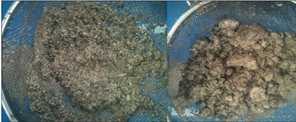
Figure 13: Cuttings Taken From the Possum Belly (Left) and at the End of the Shaker Screens (Right) (Karimi 2013)
