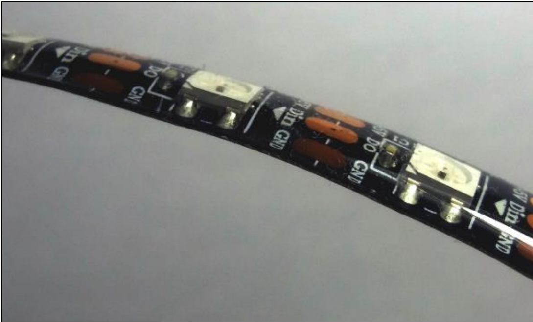
Figure 60: Example of IP 65 Protection. The Strip Is Coated with Polyurethane
