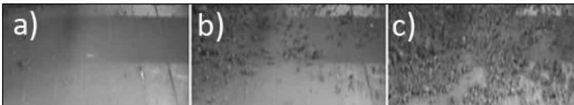
Figure 33: Images Captured by the Camera Placed Above the Shale Shakers: (a) None Concentration, (b) Low Concentration and (c) High Concentration of Cuttings (Marana, et al. 2010)
