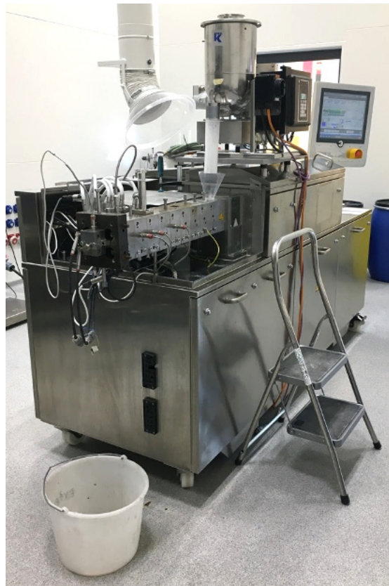
Figure 13: Coperion ZSK 18 ML with LIW feeder
