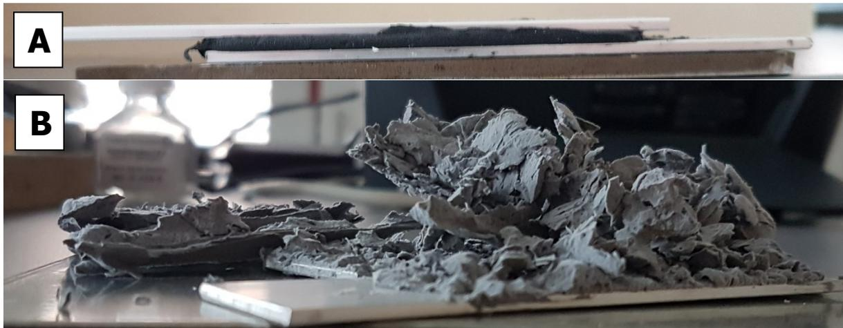
**Figure 54: Novasil filled with 50% EXP before (A) and after (B) expansion in pre-test.**
