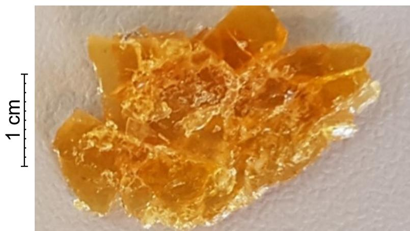
**Figure 34: DGEBA cured with SA-PDMS, catalysed by 10 mol%  $\text{Zn}(\text{AcAc})_2$  after reprocessing for 5 h at 160°C.**
