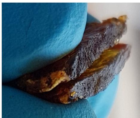
**Figure 41: Ep-PDMS cured with Pripol and reprocessed at 160°C for 5 h.**
