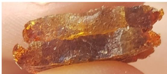
**Figure 45: Ep-PDMS cured with Pripol with TMHMDA as catalyst and reprocessed at 160°C for 5 h.**
