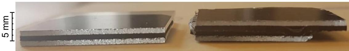
**Figure 26: Specimens filled with 30 wt.% NF and 30 wt.% EXP before (left) and after (right) expansion via inductive heating.**
