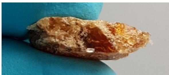
**Figure 38: Ep-PDMS cured with SA-PDMS and reprocessed at 180°C for 1 h.**
