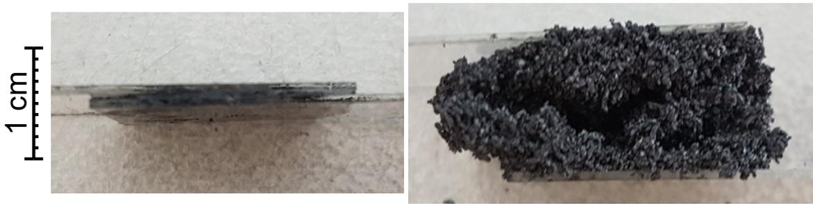
**Figure 2: Adhesive connection containing expandable graphite before (left) and after (right) expansion.**
