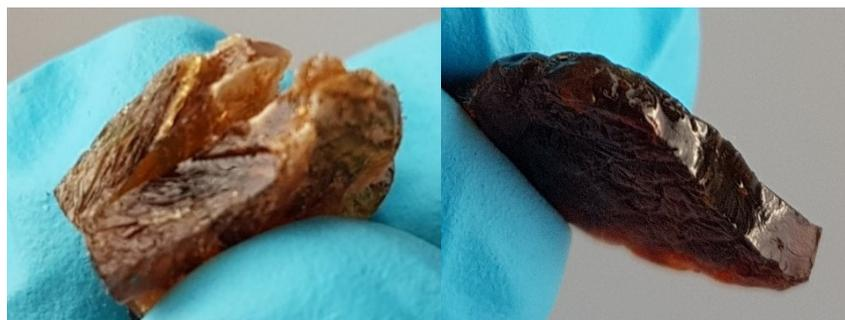
**Figure 36: Ep-PDMS cured with MHPA (left) and SA-PDMS (right) with 10 mol% Zn(AcAc)<sub>2</sub> and reprocessed at 180°C for 1 h.**
