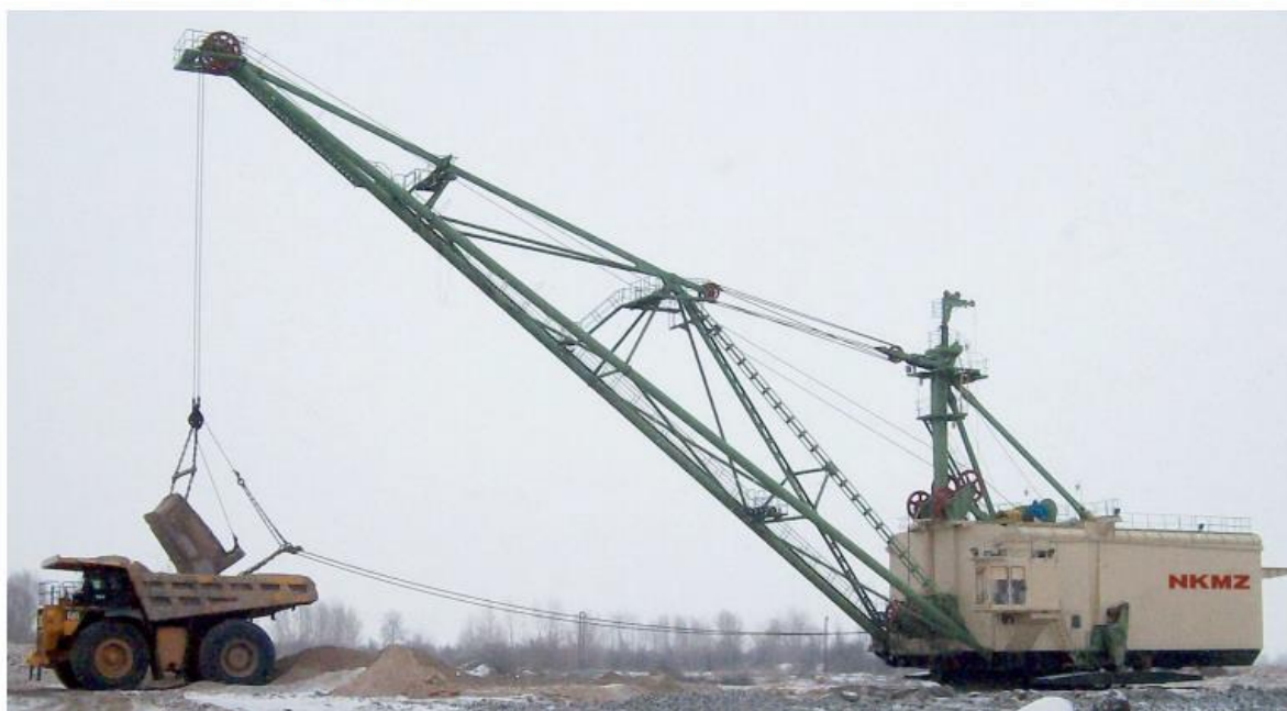
Figure 11 Scheme of aimed loading of a truck by ESh-14-50 dragline excavator [12]
