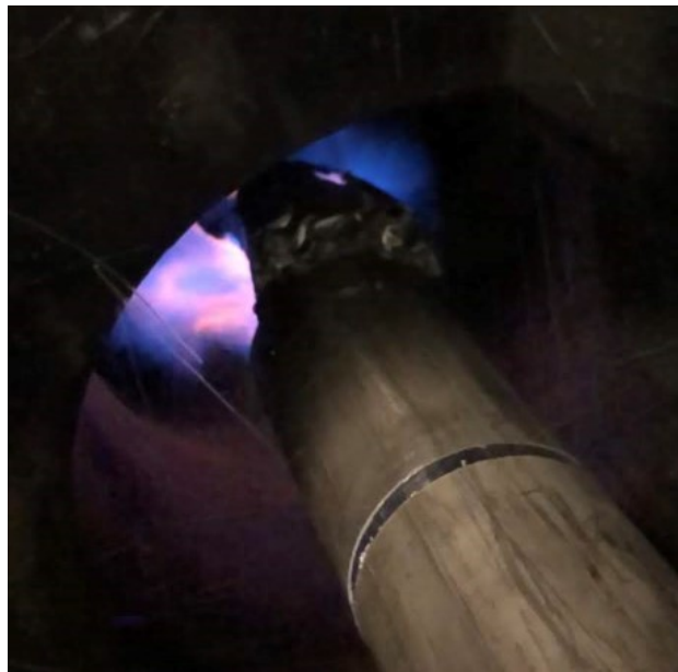
Figure 19: Image of a stoichiometric flame leaving the open-end of the steel reactor
