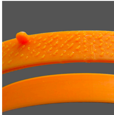
Figure 12. Visible infill from the outside.
