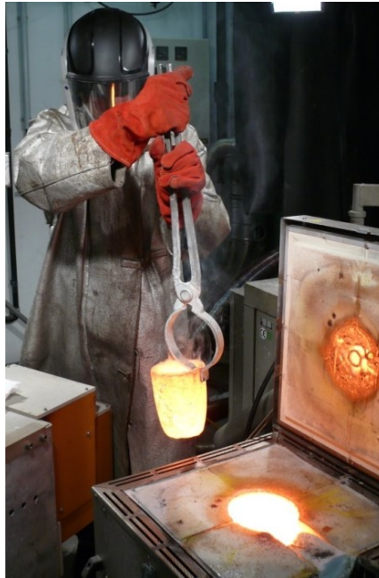
Figure 5.3: Removal of the crucible out of the furnace after finishing the trial
