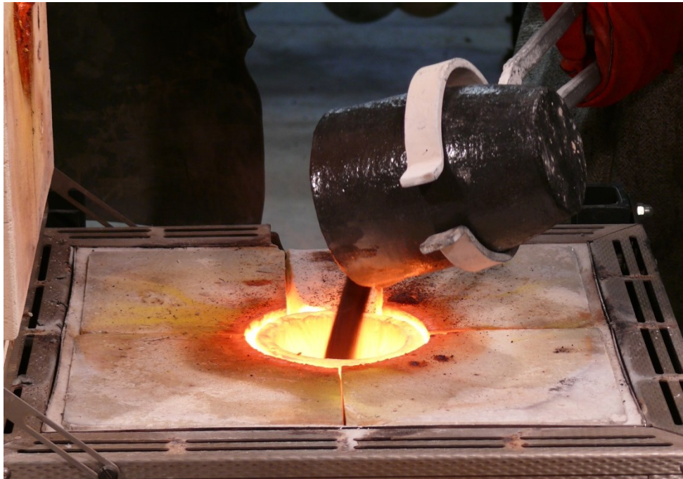
Figure 5.2: Picture of charging residue into the preheated crucible onto the lead bath
