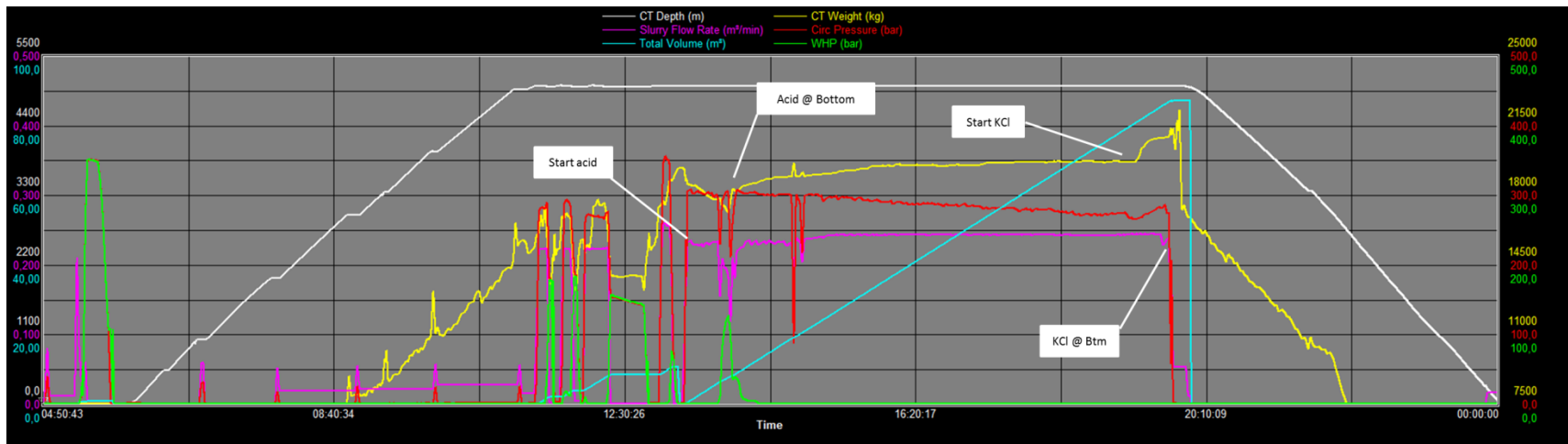
Figure A - 22: Graph treatment 5 SSD 3. The well flowing pressure was calculated with the software "Prosper".
