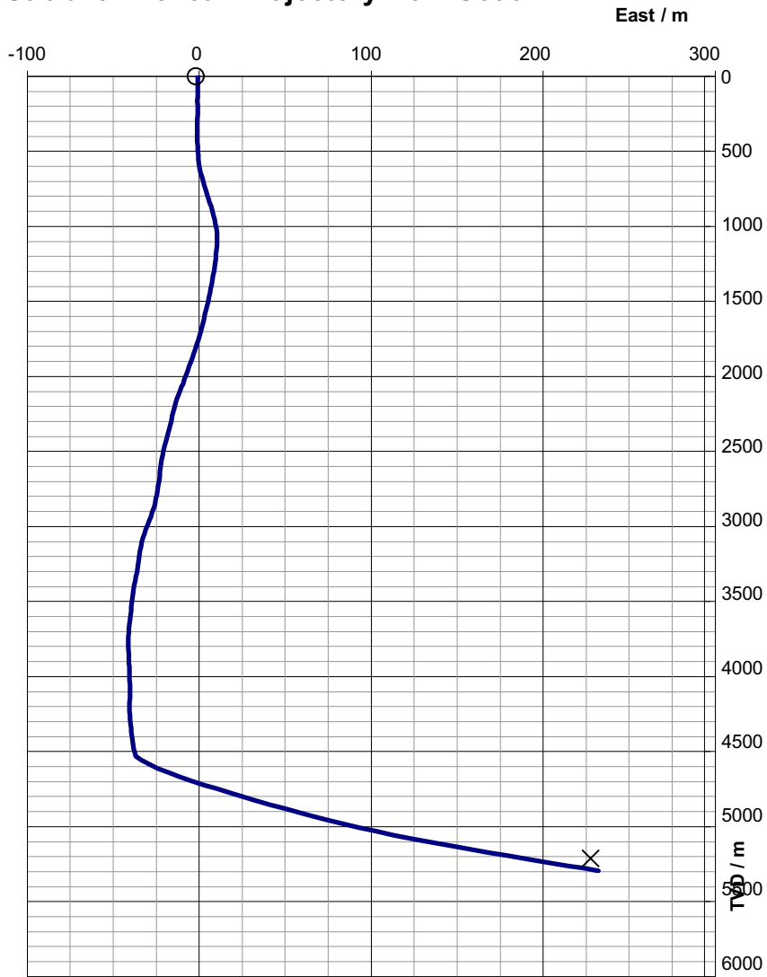
Figure A - 7: Side view from the south of the STR T 5a trajectory.
