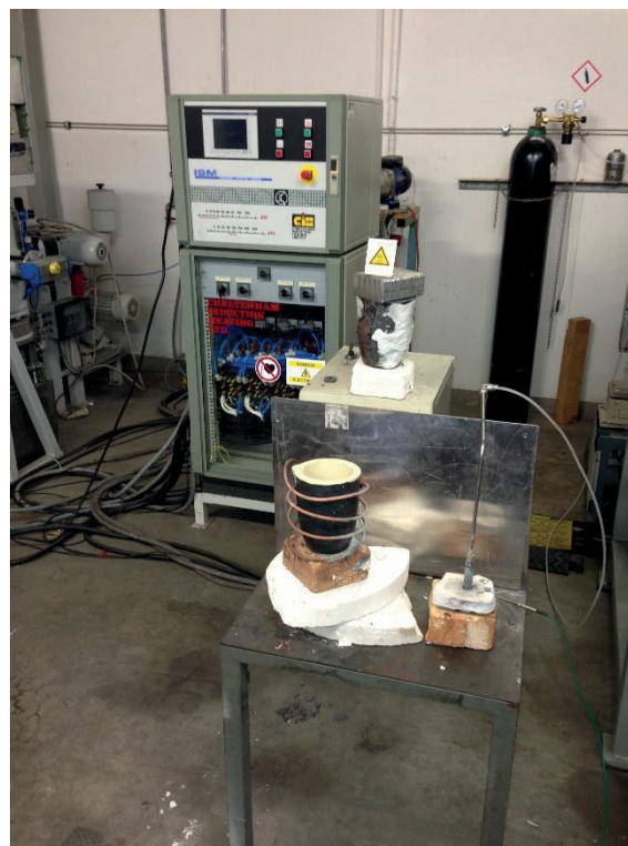
Fig. 3-3: Induction heater Cheltenham® ISM HF20, water-cooled copper coil, graphite crucible A5.
