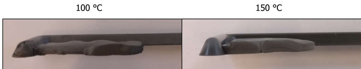
Figure 20: Tensile specimens of step 3 of the filling study at 100 \text{ }^\circ\text{C} and 150 \text{ }^\circ\text{C} mold temperature of PolyPOM FN0805 at an injection rate of 5 \text{ cm}^3/\text{s} .
