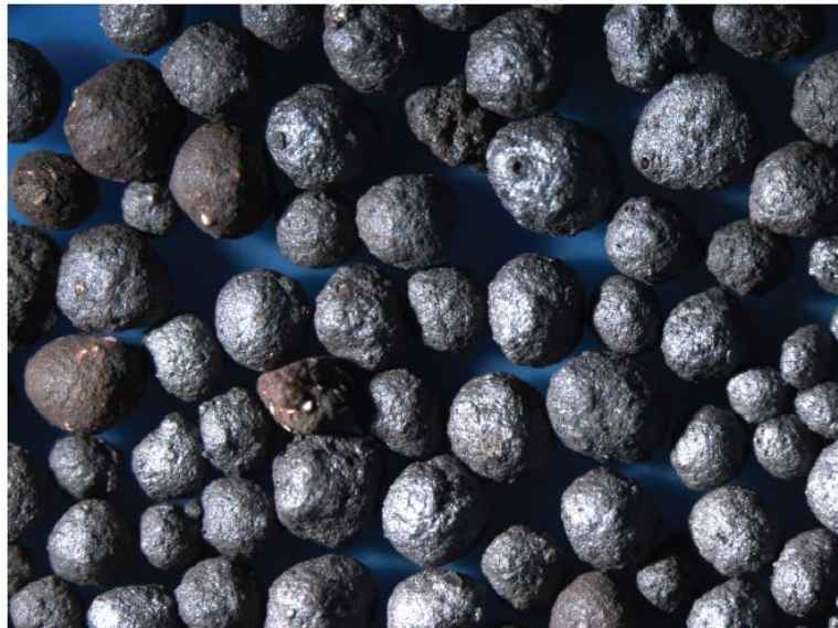
Figure 11: Sintered bauxite proppant (Economides and Martin 2007)
