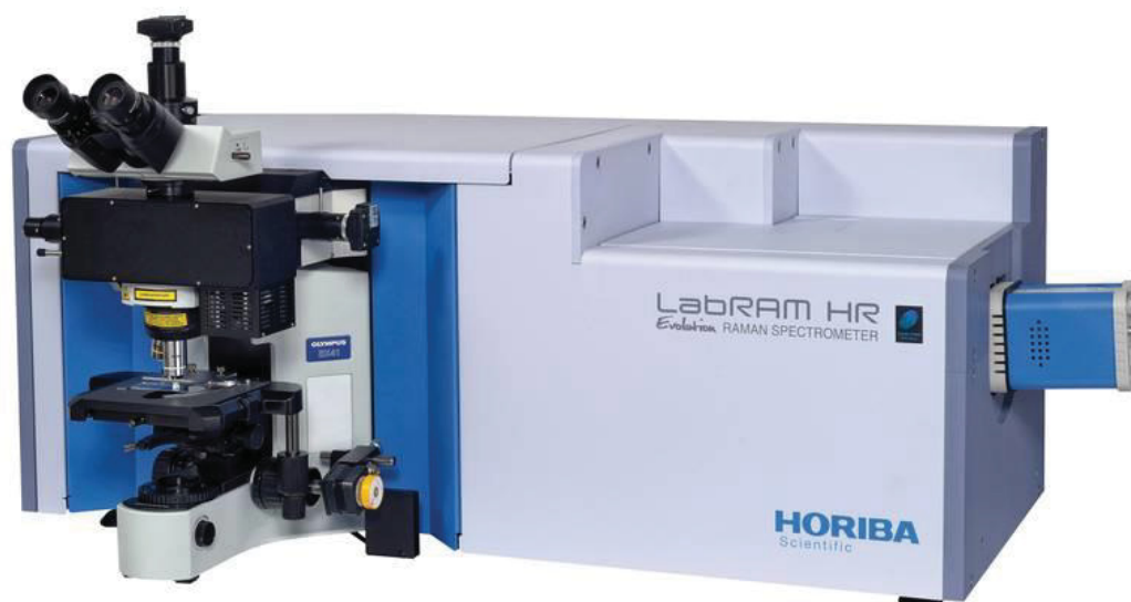
Figure 26: Picture of RAMAN set-up Horiba LabRAM HR Evolution [69].
