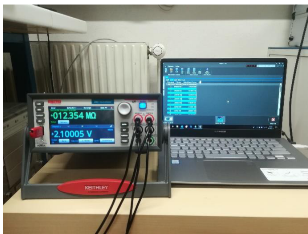
Figure 30: The SMU connected with the provided software during measurements
