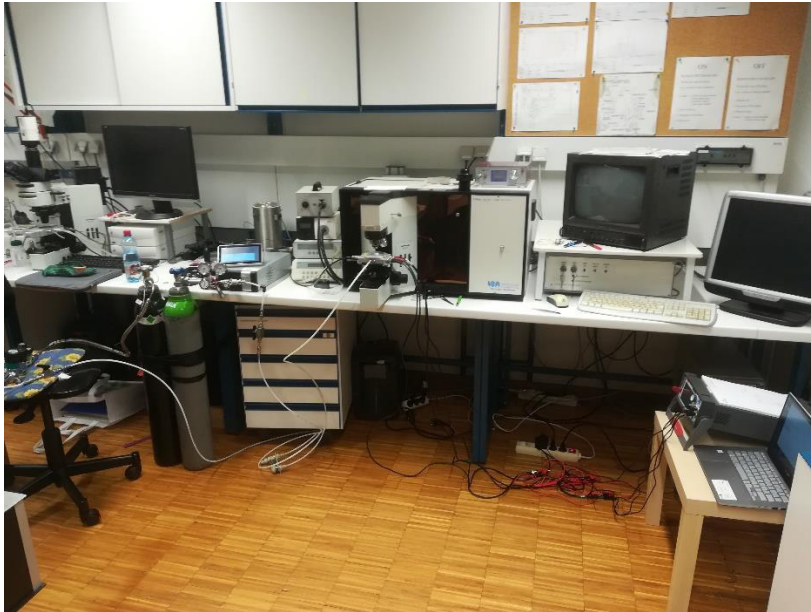
Figure 23: The in-operando gas sensing metal-oxide characterization setup with a special measurement chamber including a Raman spectrometer, gas supply, measurement chamber and electric resistance measurement
