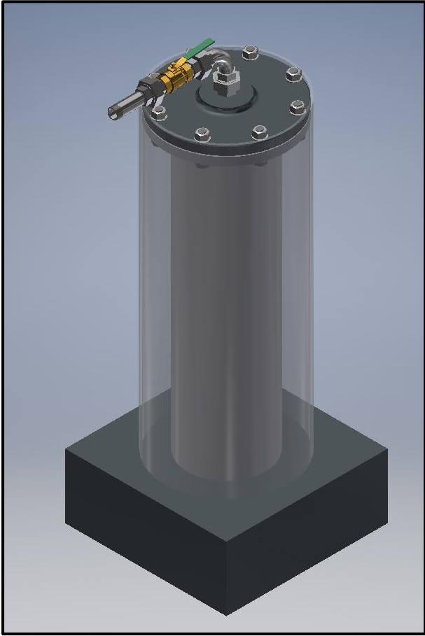
Figure 53: 3D-view of the test cell
