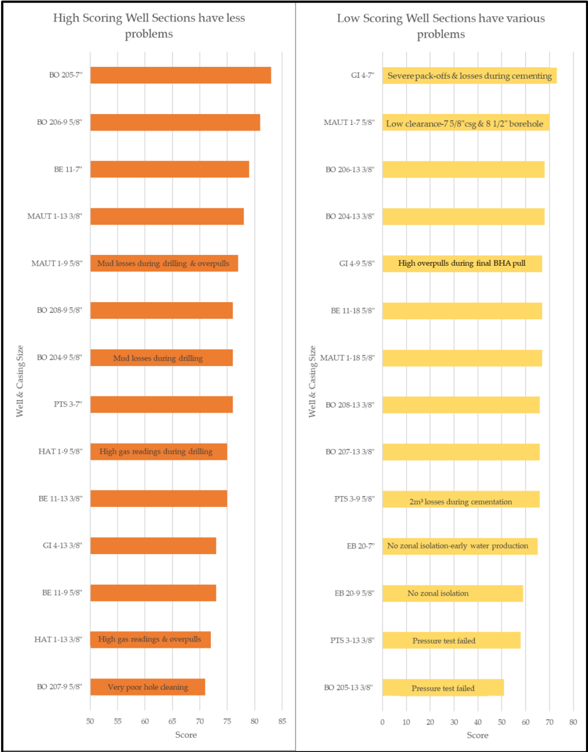
Figure 36: Summary of scores of every well section and the driving factor behind the low score
