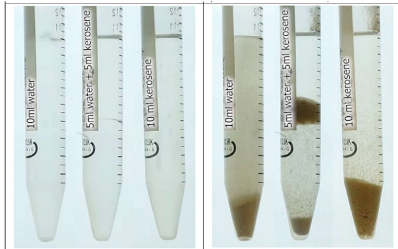
Figure 20: Sedimentation test on Kaolinite, (left): initial setup before adding kaolinite powder. 10ml of water in the left vial, 5ml of water below 5ml of kerosene in the second vial and 10ml of kerosene in the right vial. (right): Snapshot of the ongoing experiment 39 seconds after adding 0.5g of kaolinite powder to each vial
