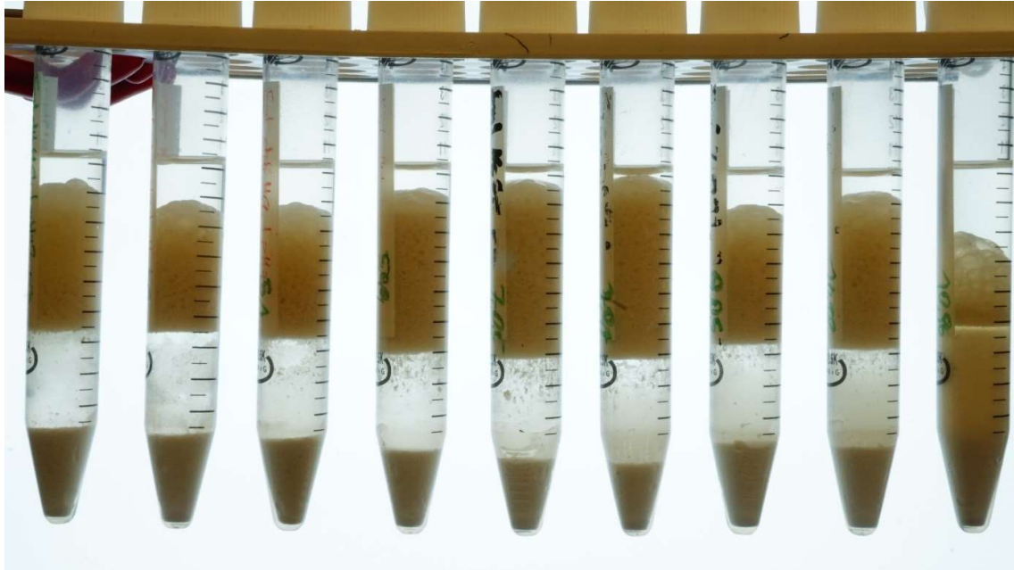
Figure 32: Emulsion Behavior of Kaolinite in 5ml of decane and 5ml of a basic and acidic solution ranging from pH=3 (left vial) to pH=11 (right vial) in steps of one pH value
