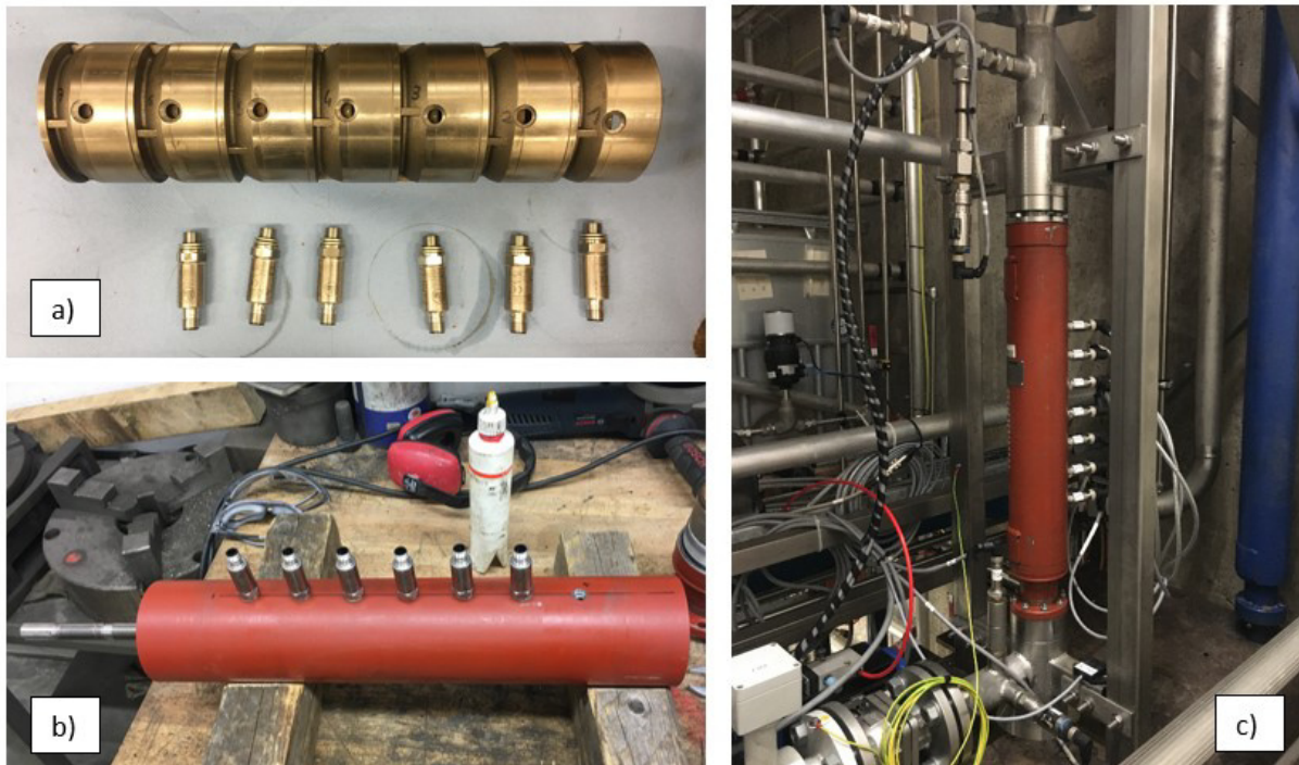
Figure 46: a) Diffusers with pressure sensing, b) Pressure sensor screwed into the pump casing, c) Pressure sensors connected to each stage of the REDA D2400N pump
