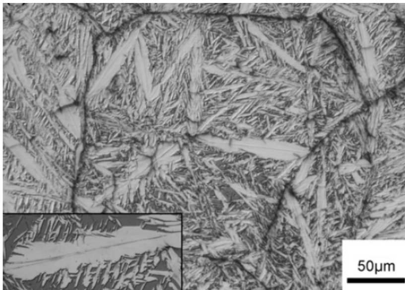
Figure 2.14: Martensitic microstructure of a Fe-1.8C (wt.-%) after solution annealing at 1200°C for 30 min and subsequent quenching in an iced brine to room temperature. The inset shows the autocatalysis of new martensitic side plates from a primary martensite plate [91].
