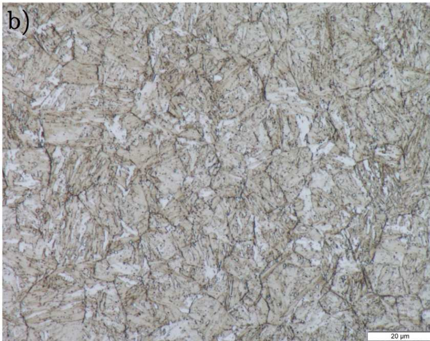
Figure 5.7: a) Evolution of volume fractions, obtained by HEXRD, of ferrite, austenite, M_2C , M_3C and M_6C during reheating of the soft annealed microstructure with 2^\circ\text{Cs}^{-1} to 1020^\circ\text{C} . b) representative optical micrograph after quenching with 100^\circ\text{Cs}^{-1} from austenitization temperature.
