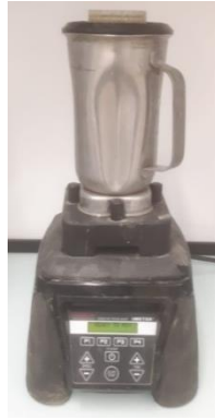
Figure 30: Constant Speed Mixer, Chandler Engineering
