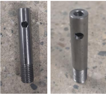
Figure 70: Cylinders to clamp fiber-optics
