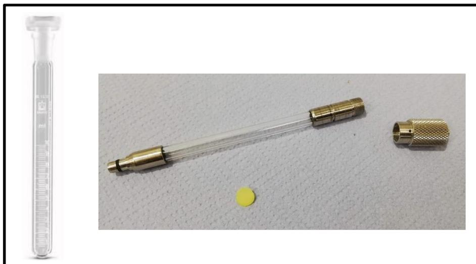
Figure 22. Testing tubes for Phase Behavior experiments, and capillary tubes for Spinning Drop Tensiometer measurements.
