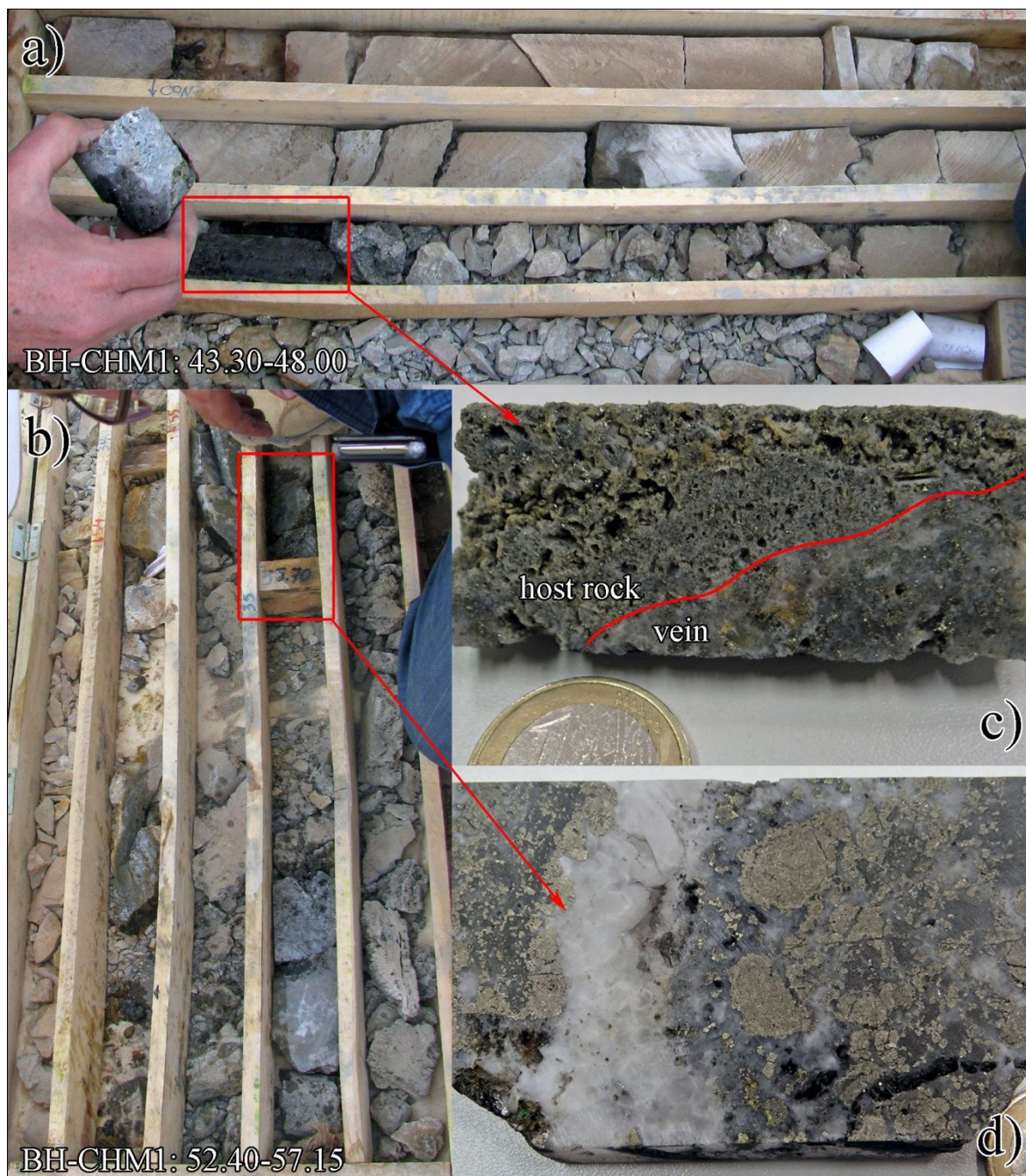
Figure 17: Massive quartz veins in drill core BH-CHM1. a) Section of drill core between 43.30-48.00 m of depth intersecting a massive 6-10 cm thick quartz vein that is surrounded by a symmetric 10-20 cm thick zone of strong silicification. Eventually, silicification grades into a zone of advanced argillic to sericitic alteration in the andesitic host rock. b) Section of drill core between 52.40-57.15 m showing strong fragmentation, which is characteristic for intersections with massive quartz veins. Several occasions of core loss are due to high decomposition of adjacent wall rocks. c) Sample CHM1-44 showing the undulating transition of a strongly silicified host rock and massive quartz vein. Voids and open spaces in the silicified host rock are due to extensive leaching of components. The dark gray part of the vein consists of disseminated sulfides in a fine-grained quartz matrix with minor amounts of carbonate. d) Massive quartz vein of sample CHM1-55.7 including nodular-shaped, polycrystalline sulfide aggregates consisting mainly of inequigranular pyrite and interstitial Cu-rich sulfides. A less mineralized band of euhedral prismatic quartz up to 1,5 cm thick is to be seen in the center.
