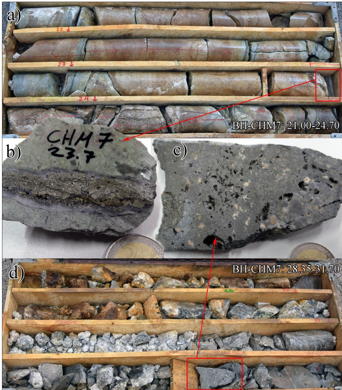
Figure 22: Photos of drill core BH-CHM7 documenting massive banded sulfide veins (so called ginguro) in altered volcanics. a) The relatively compact drill core between 21.00 and 24.70 m is dominated by greenish advanced argillic alteration adjacent to intersects of cm thick ginguro bands (e.g. at 21.20, 22.10, 23.70 m depth) and grades into sericitic alteration indicated by brownish-beige colors. b) The altered andesitic wall rock of sample CHM7-23.7 includes a 3 cm thick ginguro veinlet that is bordered by colloform bands of fine-grained quartz along the wall contact. c) Ginguro bands also occur as 10 to 20 cm thick veins of massive sulfides containing lots of voids; the light mineral is anhydrite, which has been partly leached leaving some cavities. d) Sericitic alteration (brown staining) in strongly fragmented drill core BH-CHM7 grading into a greenish-gray rock indicating advanced argillic alteration (partly silicification?) next to the ginguro vein.
