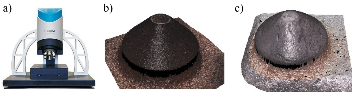
Figure 17: a) Alicona™ measurement equipment, Visualization of a b) unworn and c) worn WC/Co cemented carbide pin of a HILTI bushing tool.
