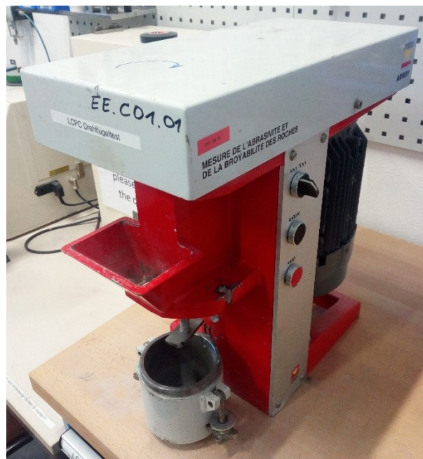
Figure 27: LCPC testing machine C.E.T.E de l'ouest, Abroy, Type 461B, No.: 39.
