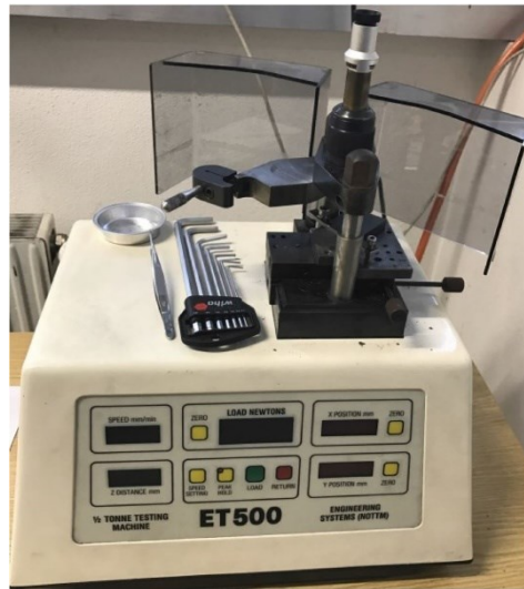
Figure 24: Edge toughness testing machine ET500
