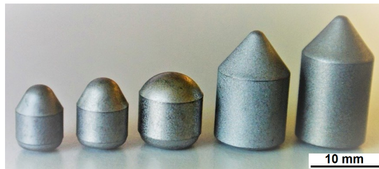
Figure 31: The different geometries of the pins for the application testing (from left to right): B2-6Co, B1-6Co, B4-9.5Co, B3-6Co and B5-9.5Co.
