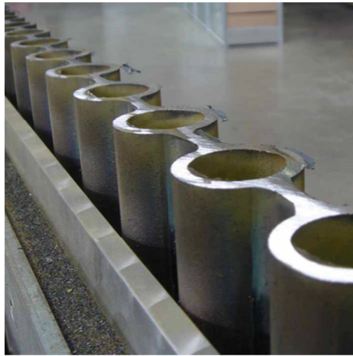
Figure 75: Detailed Picture of Membrane Wall [46]
