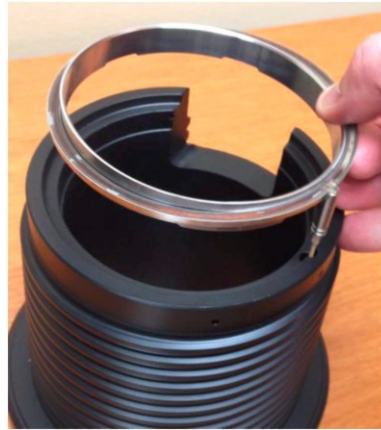
Figure 15: WDP version 2 designed to be field removable and replaceable (Sehsah et al., 2017).
