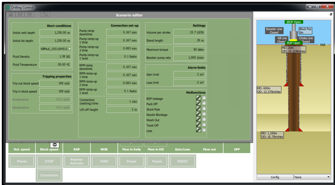
Figure 23: Drilling Control - Scenario editor
