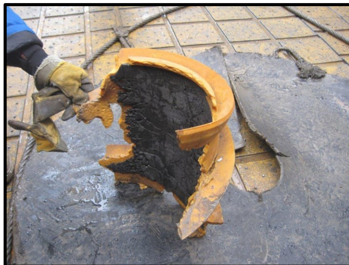
Figure 7: Junk retrieved after stuck pipe event (Cullen and Kucs 2018)
