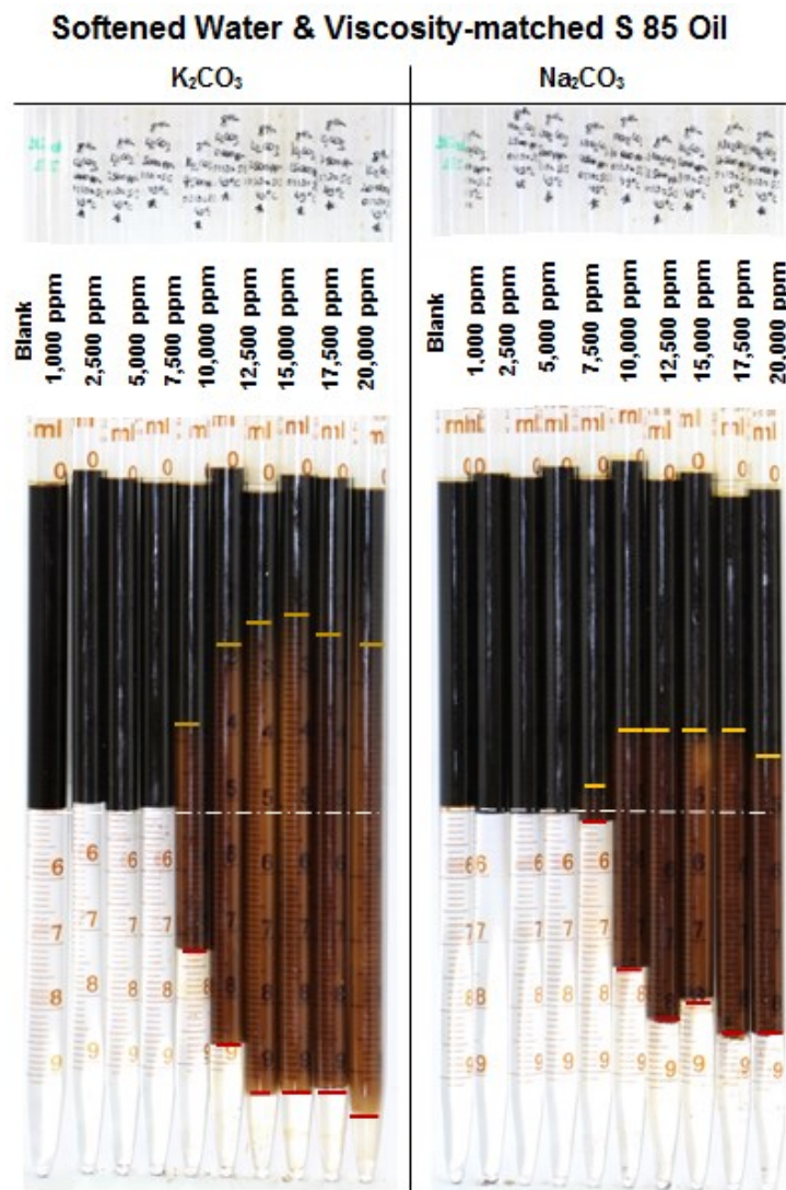
Figure 4-65: Oil scan of softened water and modified S 85 oil at 49°C for WOR 5:5 after two weeks. Yellow lines outline the oil-to-emulsion interface and the red lines the emulsion-to-water interface (Modified from [80]).
