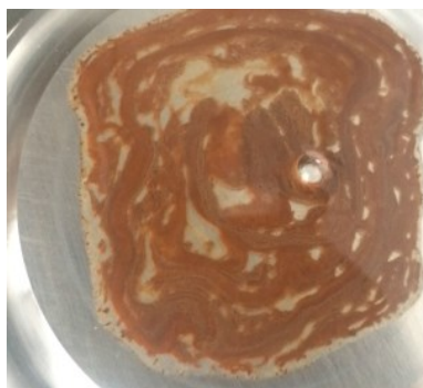
Figure 4-33: Viscosity samples of formulation 4 prepared with co-solvent 2: no stable emulsions were formed to conduct reproducible and correct viscosity measurements (separation of the emulsion phase).
