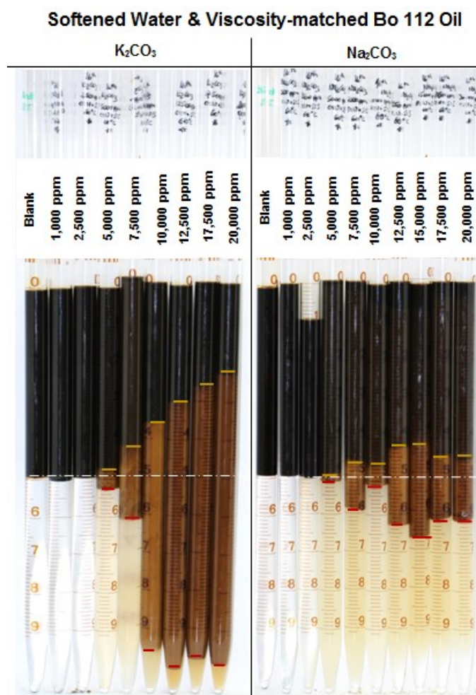
Figure 4-23: Oil scan of softened water and modified Bo 112 oil at 60°C for WOR 5:5 after two weeks. Yellow lines outline the oil-to-emulsion interface and the red lines the emulsion-to-water interface (Modified from [80]).
