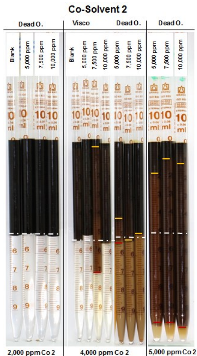
Figure 4-30: Oil scan of softened water mixed with co-solvent 2 and various alkali concentrations at 60°C for WOR 5:5 after two weeks. Yellow lines outline the oil-to-emulsion interface and the red lines the emulsion-to-water interface.
