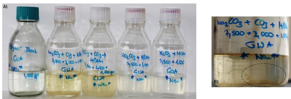
Figure 4-71: Polymer stability of the chemical formulations (A) at 60^\circ C (settling time: 2 weeks); B) precipitations of the formulations prepared with co-solvent 3.
