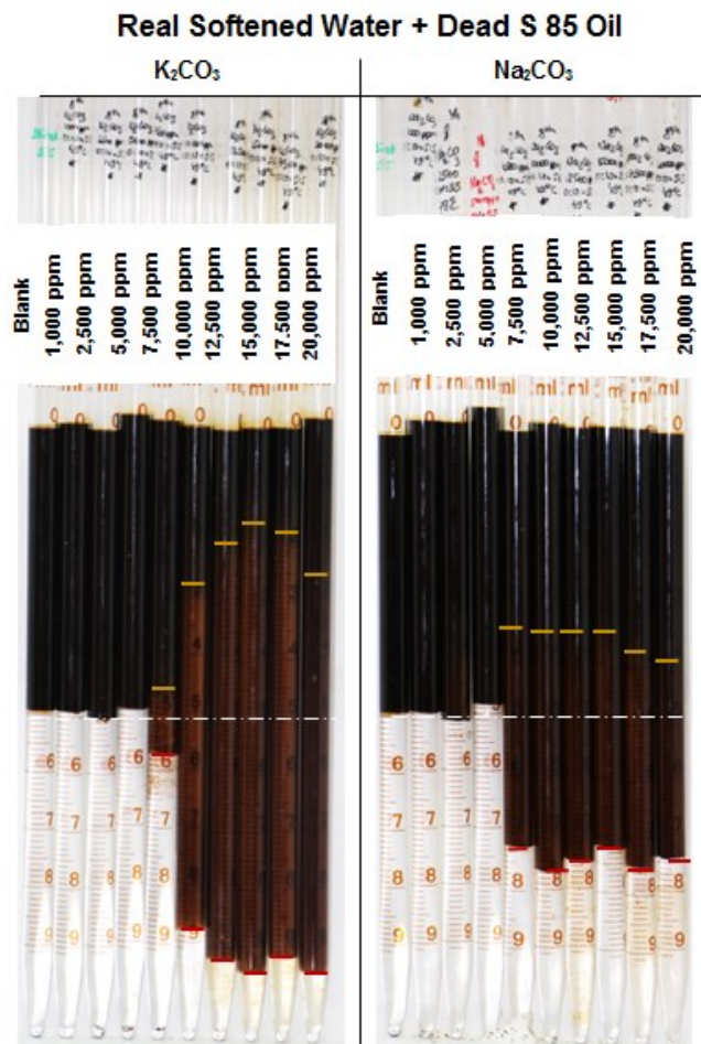
Figure 4-62: Oil scan of softened water and dead S 85 oil at 49°C after two weeks. Yellow lines outline the oil-to-emulsion interface and the red lines the emulsion-to-water interface (Modified from [80] ).
