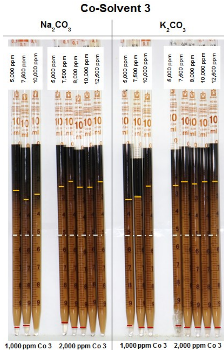
Figure 4-34: Oil scan of softened water mixed with co-solvent 3 and various alkali concentrations at 60°C for WOR 5:5 after two weeks. Yellow lines outline the oil-to-emulsion interface and the red lines the emulsion-to-water interface.
