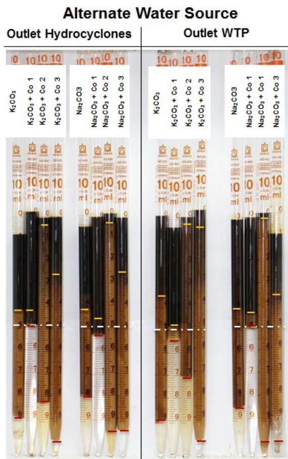
Figure 4-38: Oil scan of different types of softened water mixed with co-solvents and alkali at 60°C for WOR 5:5 after two weeks. Yellow lines outline the oil-to-emulsion interface and the red lines the emulsion-to-water interface.
